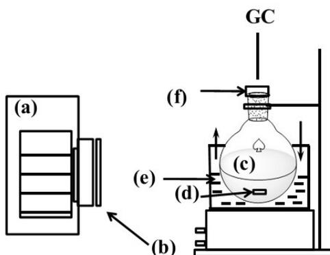
**Figure S1.** Reactor of the present photocatalytic reaction system: (a) light source of 300 W Xe lamp, (b) UV cut-off filter ( $\lambda > 420$  nm), (c) reaction solution, (d) magnetic stirring bar, (e) water jacket, (f) septum.<sup>1</sup>
