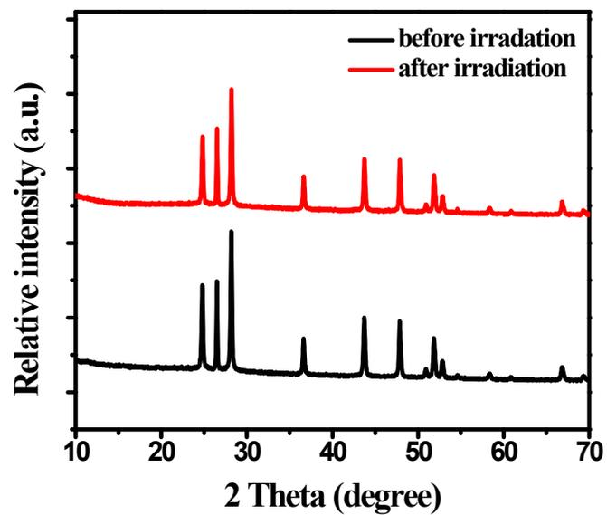
**Figure S3.** The XRD patterns of MoS<sub>2</sub>/CdS sample containing 1.52 wt% MoS<sub>2</sub> before and after 12 h photocatalytic activity under visible light irradiation ( $\lambda > 420$  nm).
