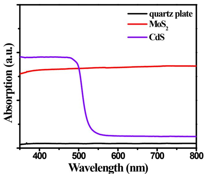
**Figure S2.** The UV-Vis spectra of the blank quartz plate, pure CdS and pure  $\text{MoS}_2$ .
