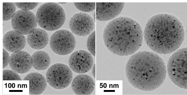
Fig. S9. TEM images of 130 nm FeCo/GC NCs@MSNs-SH after the six consecutive adsorption cycles for MO.
