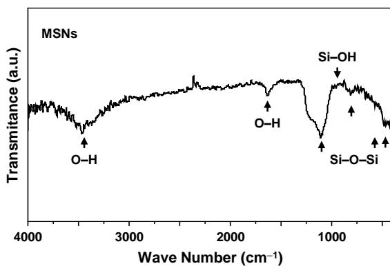
Fig. S6. FT-IR data of 130 nm MSNs.
