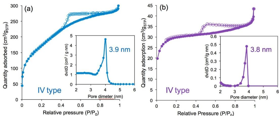
**Fig. S9.** N<sub>2</sub> adsorption-desorption isotherms and pore size distribution of the calcined of  $\mu$ -PSt-*g*-PEI/dicarboxylic acid@SiO<sub>2</sub> mediated from (a) Mucic acid, (b) Adipic acid. Open dots: desorption; close dots: adsorption.
