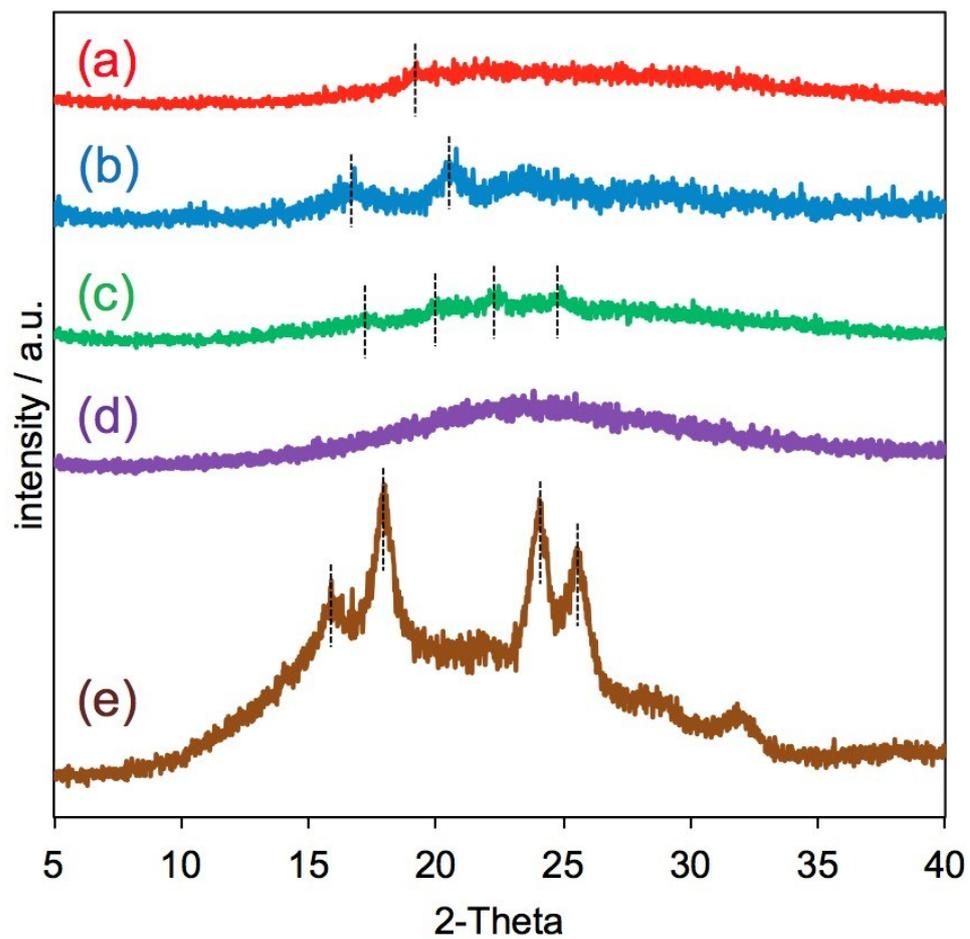
**Fig. S1.** XRD patterns of  $\mu$ -PSt-*g*-LPEI (e) and  $\mu$ -PSt-*g*-PEI/dicarboxylic acids complexes associated with m-TA (a), MA (b), SA (c) and AA (d).
