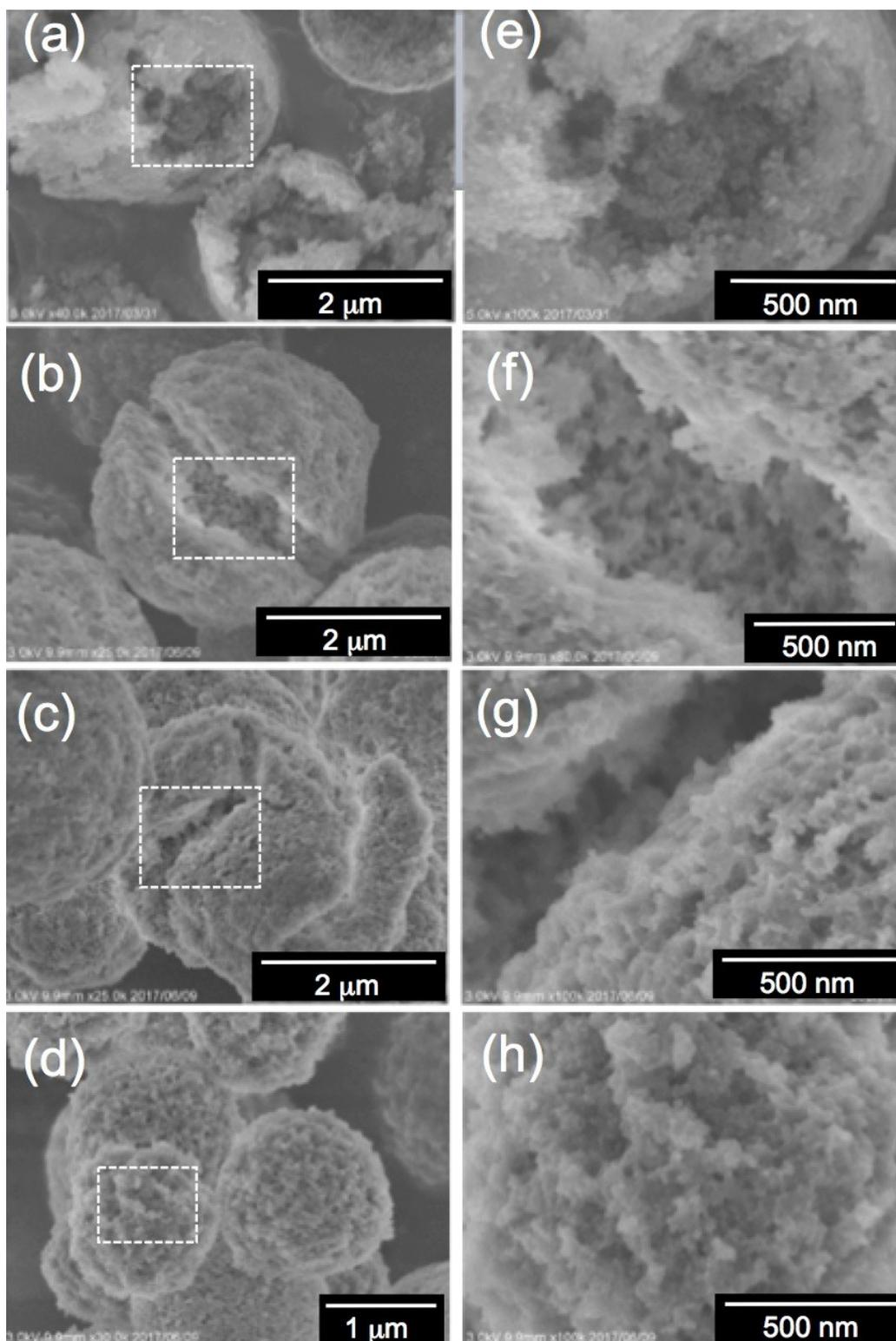
**Fig. S8.** SEM images (of magnified area) after APS treatment of calcination of  $\mu$ -PSt-g-PEI/dicarboxylic acid@SiO<sub>2</sub> mediated by different kinds of dicarboxylic acid: (a, e) m-TA, (b, f) SA, (c, g) MA, (d, h) AA.
