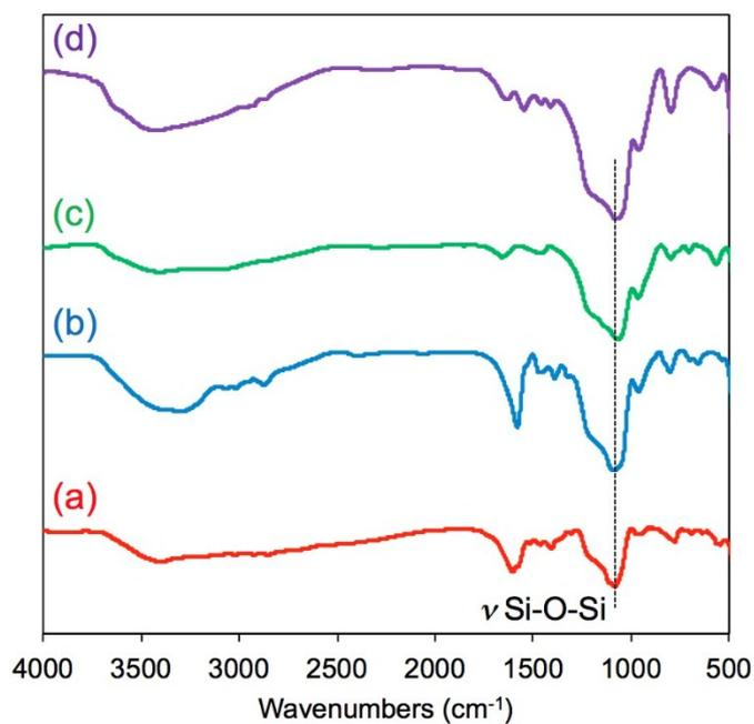
**Fig. S3.** FT-IR spectra of (a) *m*-PSt-g-PEI/*m*-TA@SiO<sub>2</sub> (b) *m*-PSt-g-PEI/MA@SiO<sub>2</sub> (c) *m*-PSt-g-PEI/SA@SiO<sub>2</sub> and (d) *m*-PSt-g-PEI/AA@SiO<sub>2</sub> .
