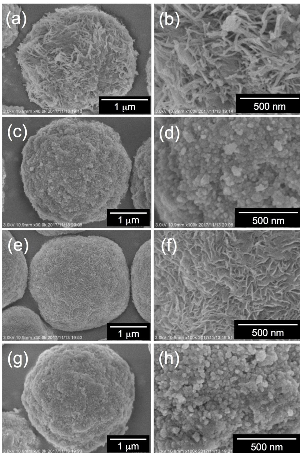
**Fig. S6.** SEM images (of magnified areas) after calcined of  $\mu$ -PSt-g-PEI/DD@SiO<sub>2</sub>. DD (dicarboxylic acid): (a, b) m-TA, (c, d) SA, (e, f) MA, (g, h) AA.
