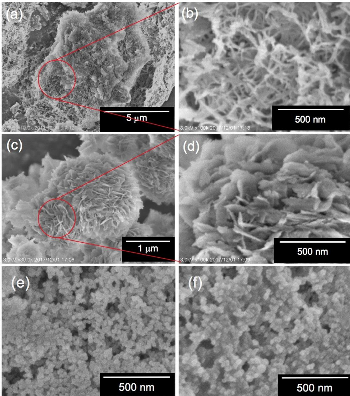
**Fig. S7.** SEM images of the silica powders templated by the complexes of cPEI/*m*-TA (a, b), cPEI/MA (c, d), cPEI/SA (e) and cPEI/AA (f). The images of (b) and (d) are the magnified observation from the red-circular areas, respectively.
