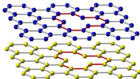
**Fig. S2** Schematic representation of a central mono-vacancy defect in both layers of the B-SNRs (mv12 configuration). Yellow balls represent atoms in the 1st layer and blue ones the atoms in the 2nd layer. Red bonds are defined in order to trace the mono-vacancy defect.
