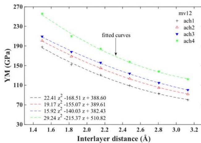
**Fig. S3** Young's modulus of mv12 defective B-SNRs configuration vs interlayer distance. ach and number label indicate the chirality and the size of the ribbon, respectively (see Table 1). Fitted curves represent the non-linear behaviour of the Young's modulus.
