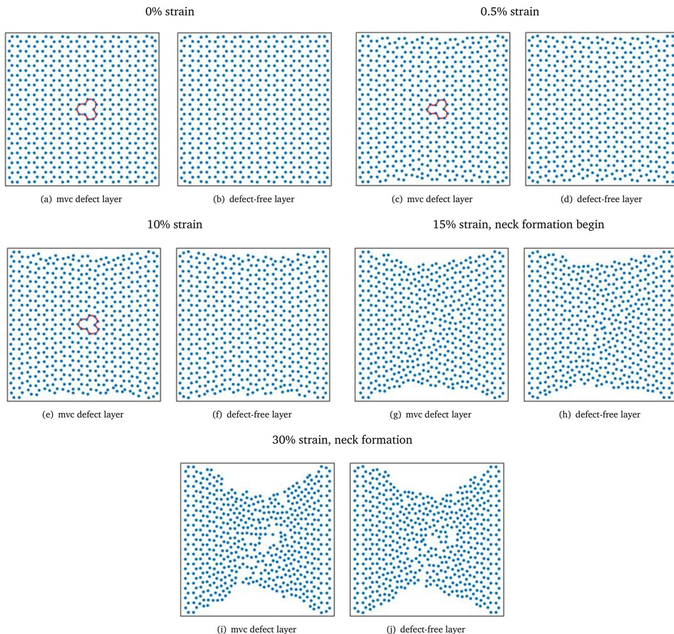
**Fig. S4** Atomic configurations for the ach3 B-SNR shown in Fig. 5 at different strains. Interlayer distance  $z=2.48$  Å. Figures on the left side correspond to the first layer and those on the right correspond to the second layer. Note that the box has been scaled along the strain direction.
