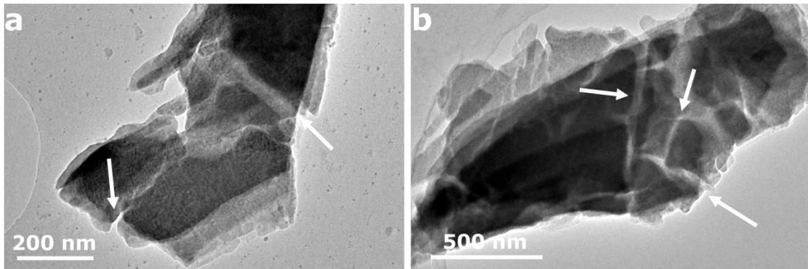
**Figure S10.** TEM characterizations of the MoS<sub>2</sub> flakes after cycling. The white arrows in both panels indicate the pulverization of flakes after repeated sodiation/desodiation.
