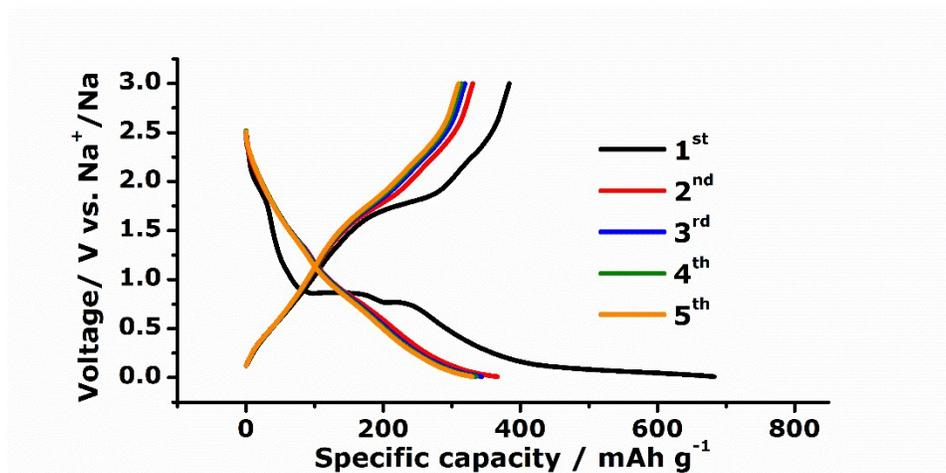
**Figure S7.** The initial galvanostatic discharge/charge curves for MoS<sub>2</sub> sample at 0.05 A g<sup>-1</sup> in the voltage range of 0.01 - 3 V.
