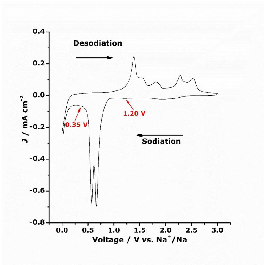
**Figure S5.** The initial CV profiles of MoS<sub>2</sub>@G hybrid measured at 0.2 mV s<sup>-1</sup> in the voltage window of 0.01 - 3 V.
