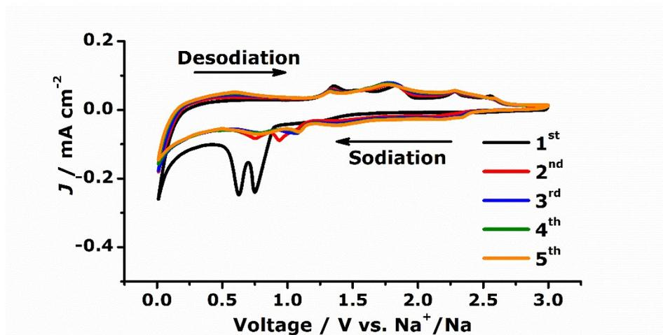
**Figure S6.** The initial CV profiles of MoS<sub>2</sub> sample measured at 0.2 mV s<sup>-1</sup> in the voltage window of 0.01 - 3 V.
