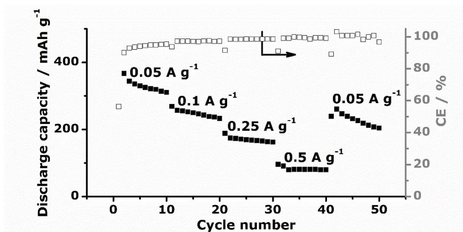
**Figure S8.** Rate performance of MoS<sub>2</sub> sample at programmed current densities.
