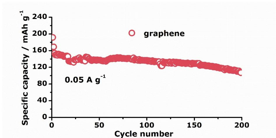
**Figure S9.** The cycling performance of graphene measured at 0.05 A g<sup>-1</sup>.
