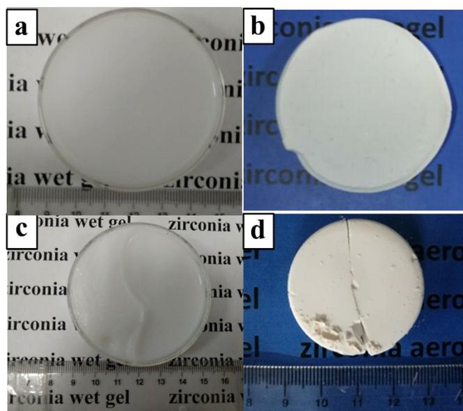
**Figure S1** Photos for the wet gel and the aerogel after supercritical drying, (a) LAA-4-wet gel, (b) LAA-4-aerogel, (c) LMA-6-wet gel and (d) LMA-6-aerogel.
