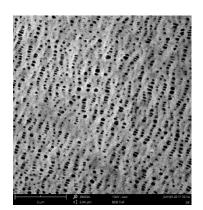
Fig. s1 SEM image of PP separator
