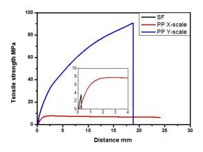
Fig. s2 the mechanical properties of SF and PP separator, X-scale is the uniaxial stretching
