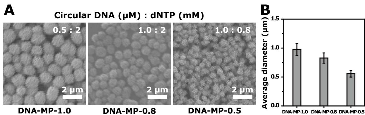
**Fig. S1** A) SEM images and B) Average diameter of CpG-based DNA-MPs including DNA-MP-0.5, DNA-MP-0.8, and DNA-MP-1.0 prepared at different circular DNA: dNTP ratios.
