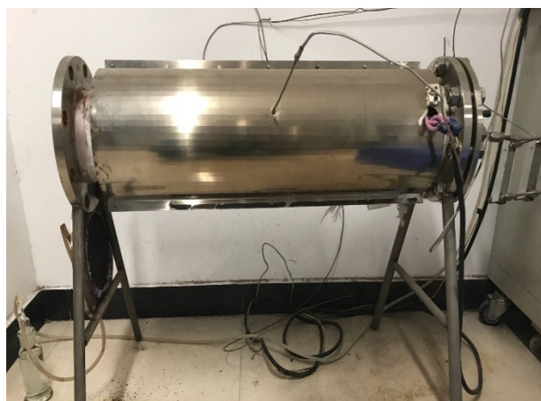
Fig. S1 the homemade tube furnace for carbonization of sodium lignosulfonate
