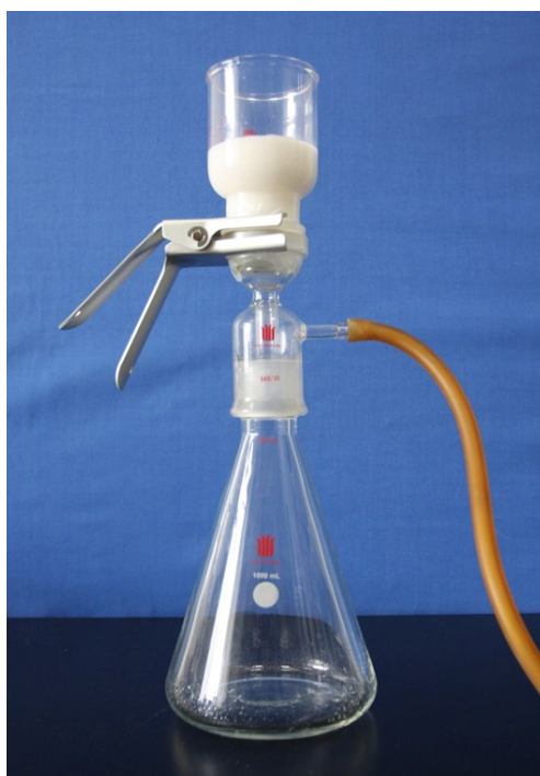
Figure S5. Photograph of the home-made filtration device. The milky-white oil-in-water emulsion is fed to the funnel, and water permeating through the membrane is collected in the flask.
