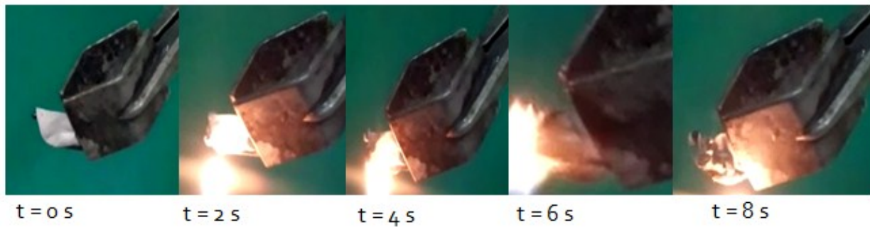
Figure S3. Combustion process of ice RS-CNTs film. The introducing of CNTs into RS enhances the flame propagation and produces severe dripping during the combustion process.
