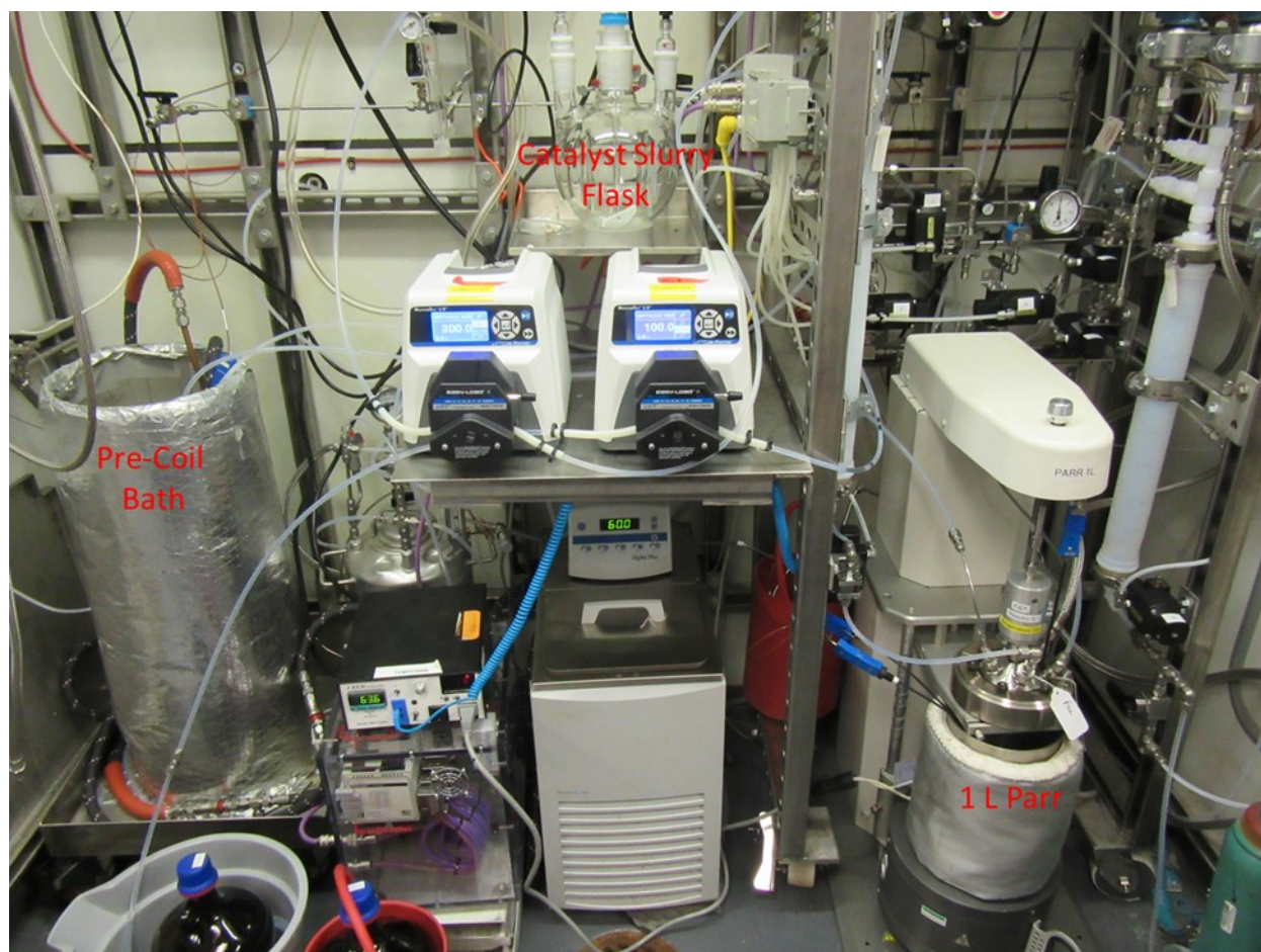
Figure 1. Picture of the 1 L Parr reactor setup in laboratory fume hood.
