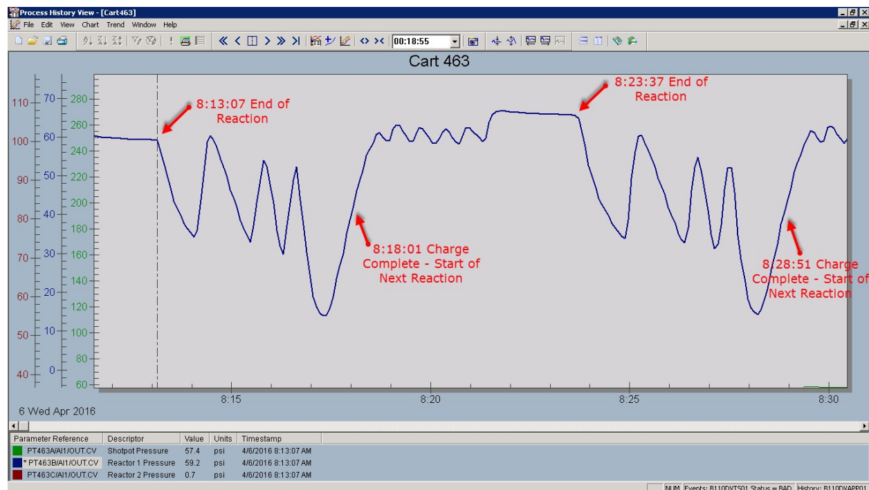
Figure 3. Reactor pressure versus time for one and a half fill-empty cycles, keeping catalyst sequestered in the reactor.
