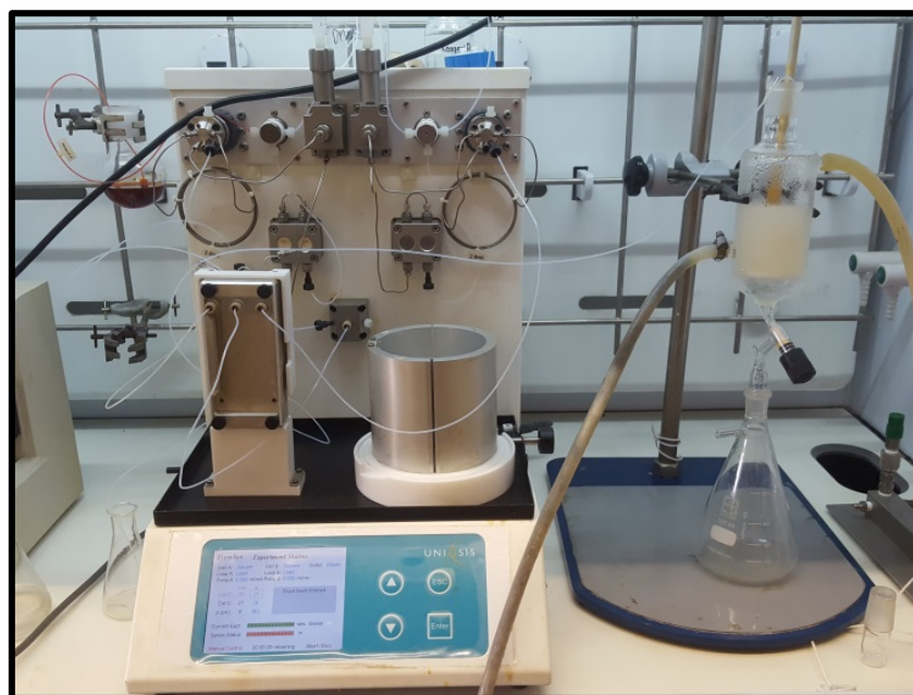
Figure 1: Reaction setup for stage 2 connected to in-line triturator
