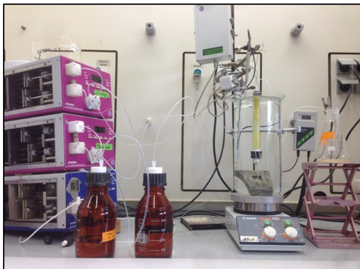
Figure 6. Experimental Setup used for the ODS of a model fuel. The syringe pumps on the left fed the model fuel and the diluted hydrogen peroxide into the tubular glass reactor dipped into a water bath.
