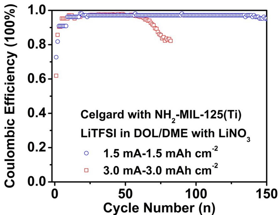
**Figure S3.** CE of Li plating/stripping under 1.5 mA cm<sup>-2</sup>-1.5 mAh cm<sup>-2</sup> and 3 mA cm<sup>-2</sup>-3 mAh cm<sup>-2</sup> conditions for Li | Cu cells with the NH<sub>2</sub>-MIL-125(Ti)-coated separator.
