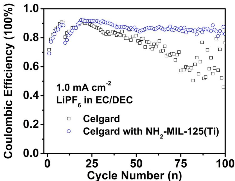
**Figure S5.** CE of Li plating/stripping under  $1 \text{ mA cm}^{-2}$ - $1 \text{ mAh cm}^{-2}$  conditions for Li | Cu cells with the pristine and  $\text{NH}_2\text{-MIL-125(Ti)}$ -coated separators. The electrolyte is  $1.0 \text{ M LiPF}_6$  in mixed EC/DEC (1:1 V/V). The cells were first conditioned at  $0.25 \text{ mA cm}^{-2}$ - $0.25 \text{ mAh cm}^{-2}$  for 10 cycles before entering  $1 \text{ mA cm}^{-2}$ - $1 \text{ mAh cm}^{-2}$  cycling.
