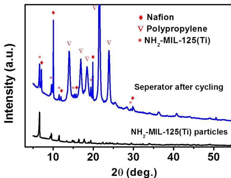
**Figure S8.** XRD pattern of the NH<sub>2</sub>-MIL-125(Ti)-coated separator after repeated lithium
