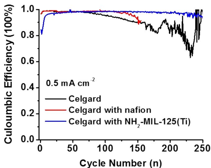
**Figure S11.** CE of consecutive Li plating/stripping cycles under 0.5 mA cm<sup>-2</sup>-1.0 mAh cm<sup>-2</sup> conditions for Li | Cu cells with the pristine separator, a Nafion-coated separator, and the NH<sub>2</sub>-MIL-125(Ti)-coated separator.
