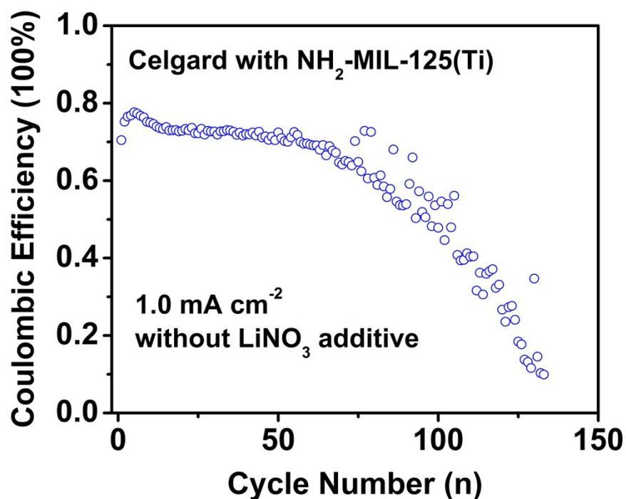
**Figure S4.** CE of Li plating/stripping under 1 mA cm<sup>-2</sup>-1 mAh cm<sup>-2</sup> conditions for a Li | Cu cell with the NH<sub>2</sub>-MIL-125(Ti)-coated separator but without LiNO<sub>3</sub> additive in the electrolyte.
