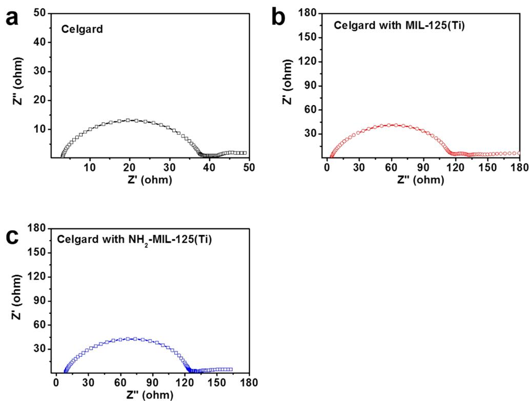
**Figure S10.** EIS spectra of Li | Li cells with the (a) pristine, (b) MIL-125 (Ti)-coated and (c) NH<sub>2</sub>-MIL-125 (Ti)-coated separators.
