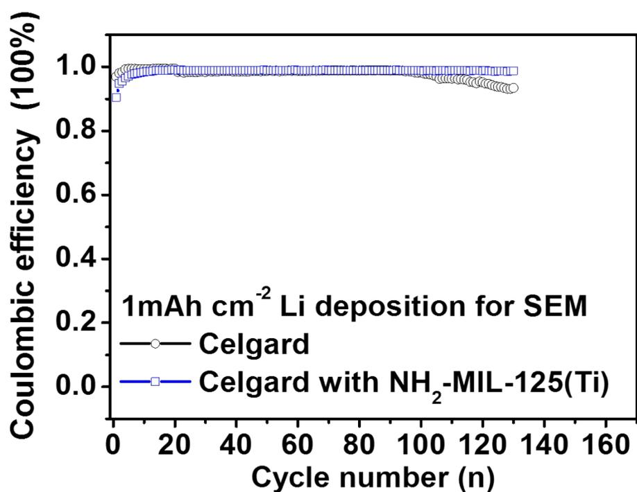
**Figure S7.** CE of consecutive Li plating/stripping cycles under 0.5 mA cm<sup>-2</sup>-1 mAh cm<sup>-2</sup> conditions for Li | Cu cells with the pristine and NH<sub>2</sub>-MIL-125(Ti)-coated separators. The electrodes after cycling were imaged with SEM to generate the results shown in Figure 4. The separator after cycling was analyzed with XRD to get the diffraction pattern in Figure S8.
