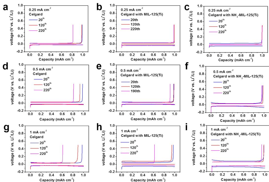
**Figure S9.** Discharging and charging voltage profiles of Li | Cu cells with the pristine (a, d and g), MIL-125 (Ti)-coated (b, e and h) and  $\text{NH}_2\text{-MIL-125 (Ti)}$ -coated (c, f and i) separators at various current densities of 0.25, 0.5 and 1  $\text{mA cm}^{-2}$ .
