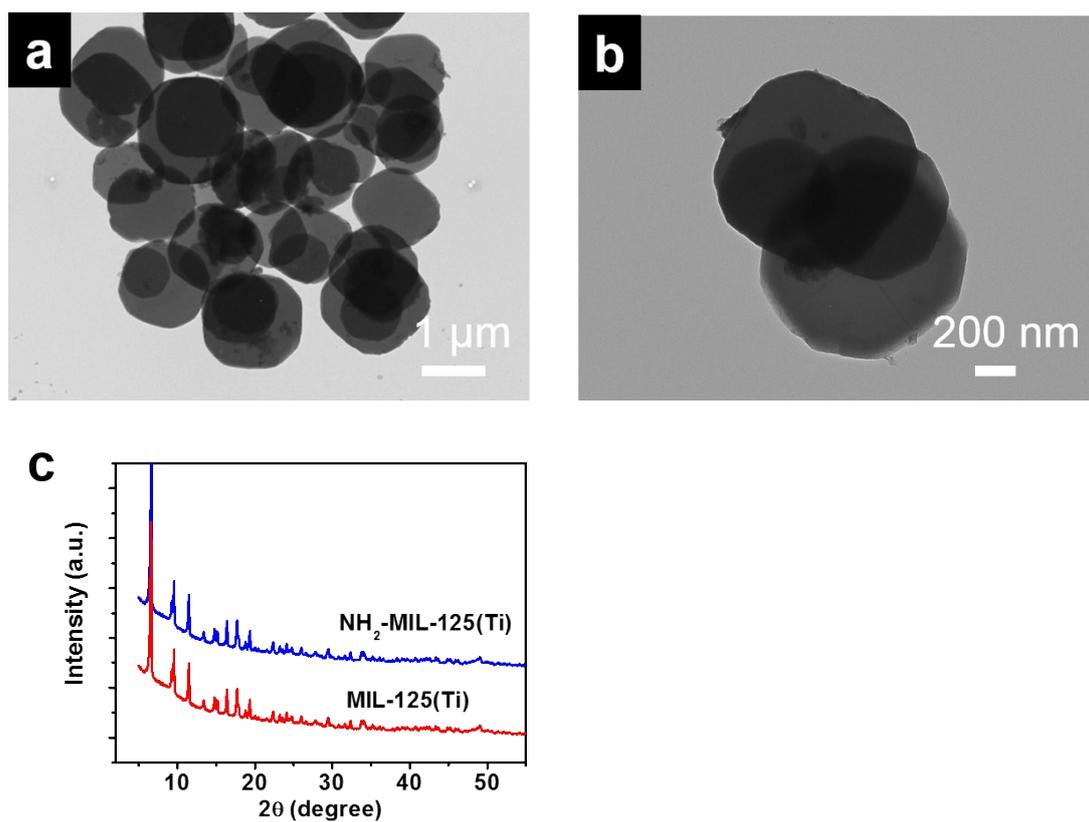
**Figure S2.** (a, b) TEM images of synthesized NH<sub>2</sub>-MIL-125(Ti). (c) XRD patterns of MIL-125(Ti) and NH<sub>2</sub>-MIL-125(Ti).
