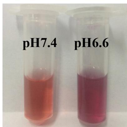
**Fig. S1** Photograph of the GNMs at pH 7.4 and 6.6 in PBS buffer. The colour changes from burgundy in neutral pH to dark-violet in mildly acidic conditions.
