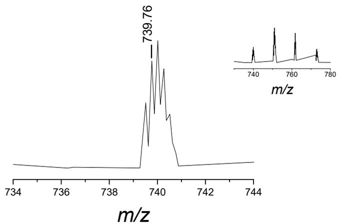
**Figure 28g.** Mass spectrum of  $[4+2d]$  (0.35 kDa) produced in borate buffer. HRMS (ESI-ion trap)  $m/z$ : Parent ions:  $[M + 4H]^{4+}$  Calcd for  $\frac{1}{4} \times C_{141}H_{212}ClN_{27}O_{38}S^{4+}$  739.87 (Found: 739.76).
