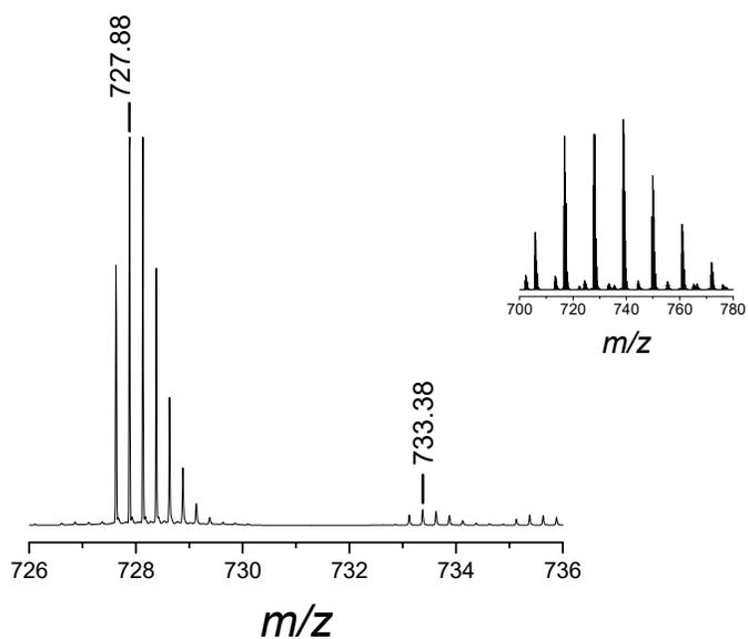
**Figure 28e.** Mass spectrum of [4+2c] (0.35 kDa) produced in borate buffer. . HRMS (ESI-ion trap) m/z: Parent ions:  $[M + 4H]^{4+}$  Calcd for  $\frac{1}{4} \times C_{140}H_{211}N_{27}O_{38}S^{4+}$  727.88 (Found: 727.88);  $[M + 3H + Na]^{4+}$  Calcd for  $\frac{1}{4} \times C_{142}H_{214}N_{27}NaO_{38}S^{4+}$  733.37 (Found: 733.38).
