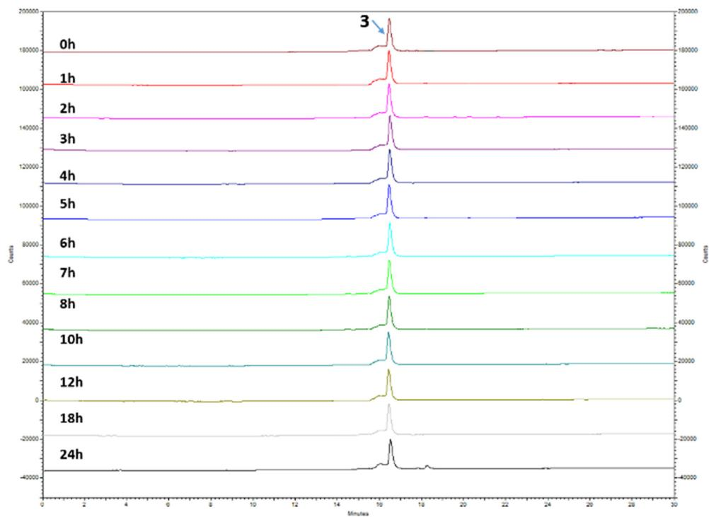
**Figure S23.** Representative HPLC chromatograms (fluorescence) of the PEGylation of **3** with **2d** (0.35 kDa).
