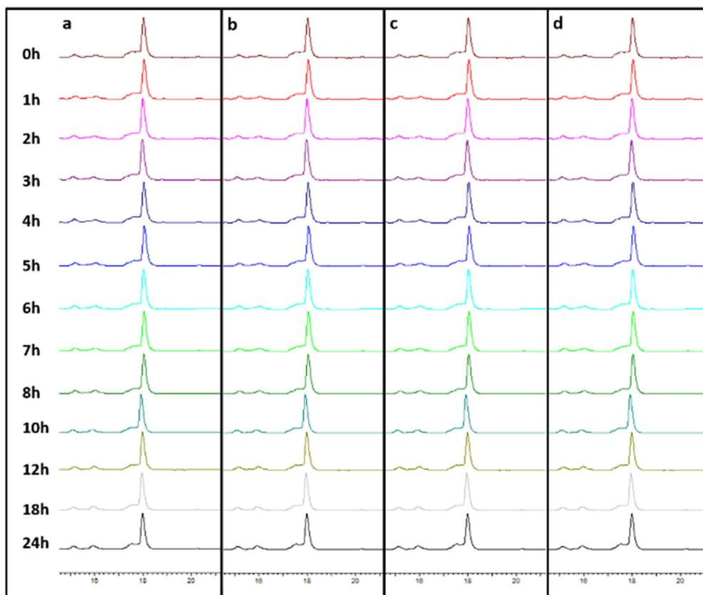
**Figure S24.** Representative HPLC chromatograms (fluorescence) of the PEGylation process of **5** with **2a** (a), **2d** (b), **2c** (c), or **2b** (d) (0.35 kDa). Because **5** does not possess arginine residues, no evolution of the chromatograms is observed.
