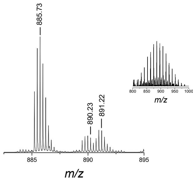
**Figure 28h.** Mass spectrum of **[4+2a]** (1 kDa) produced in borate buffer. HRMS (ESI-ion trap) m/z: Parent ions:  $[M + 4H]^{4+}$  Calcd for  $\frac{1}{4} \times C_{169}H_{269}N_{27}O_{52}S^{4+}$  885.72 (Found: 885.73);  $[M + 3H + Na]^{4+}$  Calcd for  $\frac{1}{4} \times C_{169}H_{268}N_{27}NaO_{52}S^{4+}$  891.22 (Found: 891.22);  $[M + 4H + H_2O]^{4+}$  Calcd for  $\frac{1}{4} \times C_{169}H_{271}N_{27}O_{53}S^{4+}$  890.22 (Found: 890.23).
