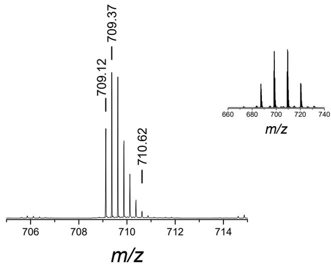
**Figure S28b.** Mass spectrum of **[4+2a]** (0.35 kDa) produced in borate buffer. HRMS (ESI-ion trap)  $m/z$ : Parent ions:  $[M + 4H]^{4+}$  Calcd for  $\frac{1}{4} \times C_{137}H_{205}N_{27}O_{36}S^{4+}$  709.37 (Found: 709.37).
