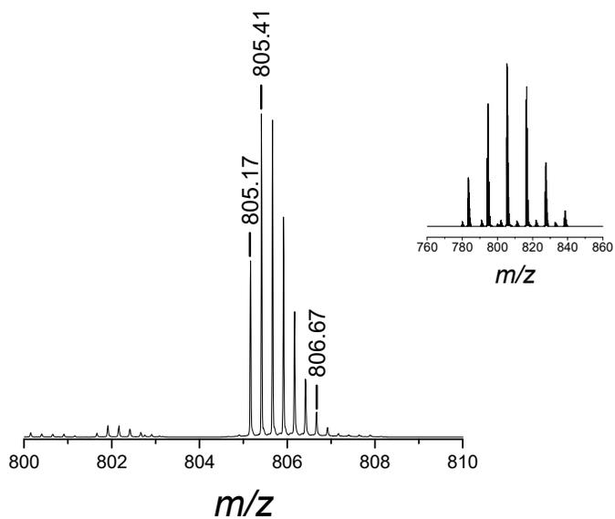
**Figure S28c.** Mass spectrum of **[4+(2a)<sub>2</sub>]** (0.35 kDa) produced in borate buffer. HRMS (ESI-ion trap)  $m/z$ : Parent ions:  $[M + 4H]^{4+}$  Calcd for  $\frac{1}{4} \times C_{156}H_{233}N_{27}O_{44}S^{4+}$  805.41 (Found: 805.41).
