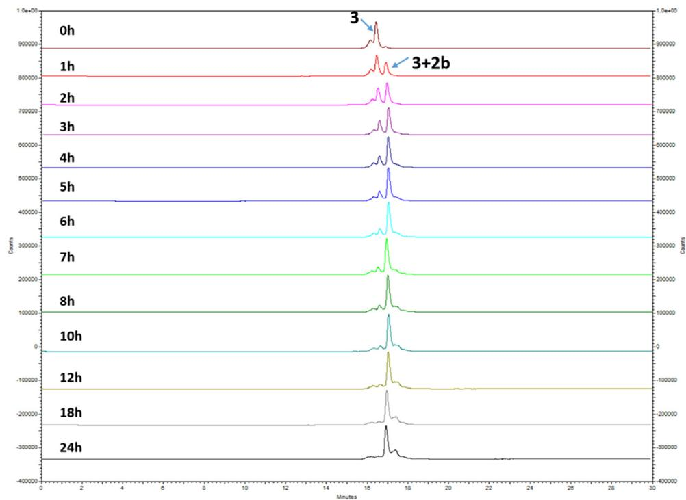
**Figure S21.** Representative HPLC chromatograms (fluorescence) of the PEGylation of **3** with **2b** (0.35 kDa).
