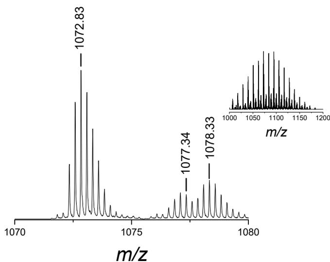
**Figure 28i.** Mass spectrum of **[4+2a]** (2 kDa) produced in borate buffer. HRMS (ESI-ion trap) m/z: Parent ions:  $[M + 4H]^{4+}$  Calcd for  $\frac{1}{4} \times C_{203}H_{337}N_{27}O_{69}S^{4+}$  1072.84 (Found: 1072.83);  $[M + 3H + Na]^{4+}$  Calcd for  $\frac{1}{4} \times C_{203}H_{336}N_{27}NaO_{69}S^{4+}$  1078.33 (Found: 1078.33);  $[M + 4H + H_2O]^{4+}$  Calcd for  $\frac{1}{4} \times C_{203}H_{339}N_{27}O_{70}S^{4+}$  1077.34 (Found: 1077.34).
