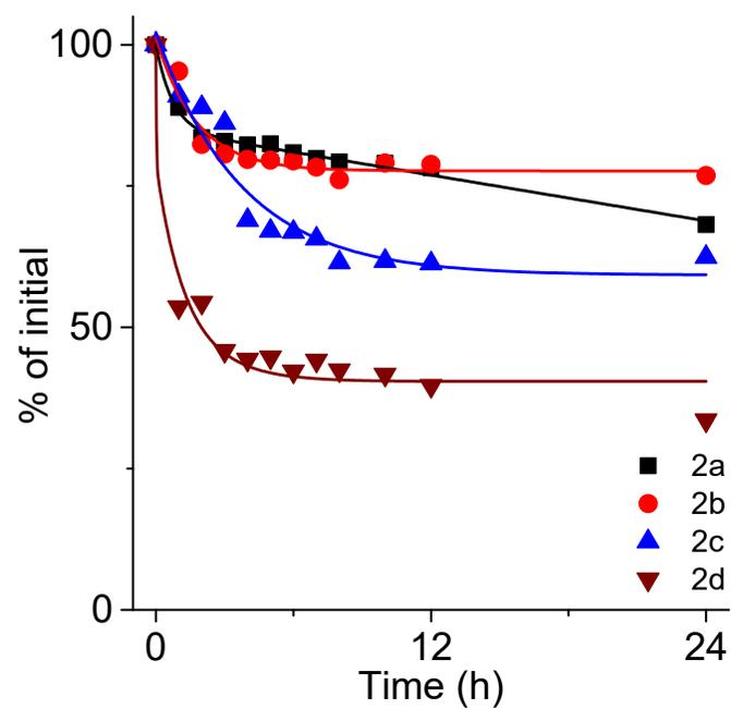
**Figure S26.** Reaction of cysteine with 1 eq. of **2a–d** (0.35 kDa) in 100 mM phosphate buffer pH 7.4 over 24 h ( $n = 1$ ). These reactions are incomplete and plateau because of the oxidation of cysteine to cystine.
