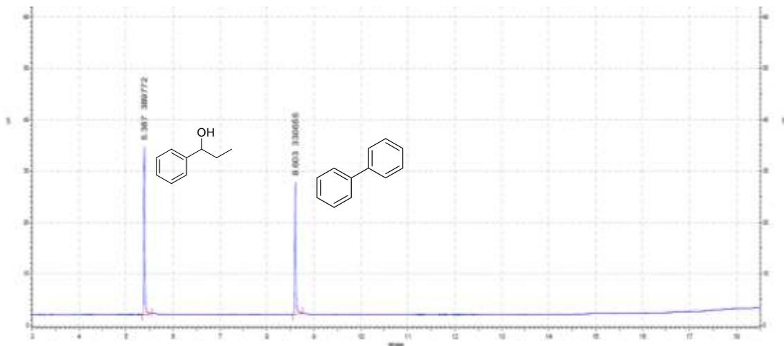
Figure SI.2.101. GC-FID chromatogram of the reduced product **10b** from the catalysis.
