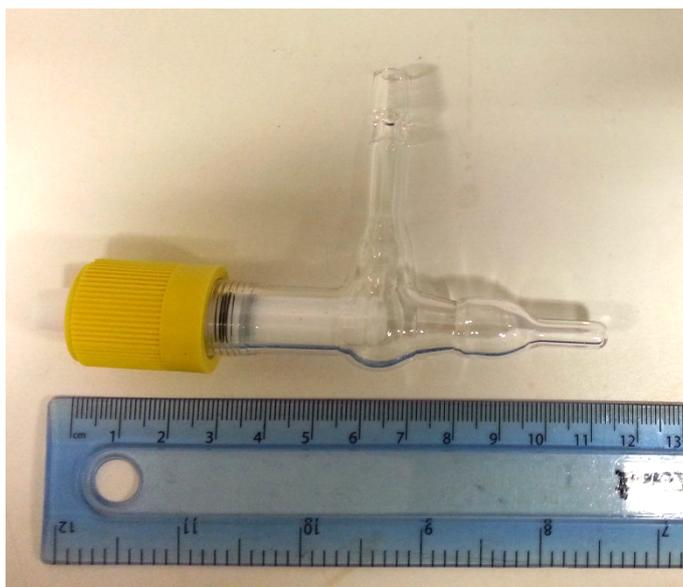
**Figure S1:** Custom built glassware for capping a solid state NMR rotor under a flush of reagent gas.
