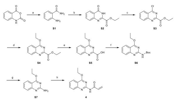
Reagents and conditions: (a) NH<sub>3</sub> in MeOH; (b) diethyl oxalate, 180 °C (2 steps, 43%); (c) SOCl<sub>2</sub>, (cat)DMF, CHCl<sub>3</sub>, reflux; (d) EtONa, EtOH, rt (2 steps, 71%); (e) 2M NaOH, EtOH, rt; (f) DPPA, Et<sub>3</sub>N, tBuOH, reflux (2 steps, 48%); (g) TFA, CH<sub>2</sub>Cl<sub>2</sub>, rt (quant); (h) Acryloyl chloride, KHMDS, THF, 0 °C (36%).
