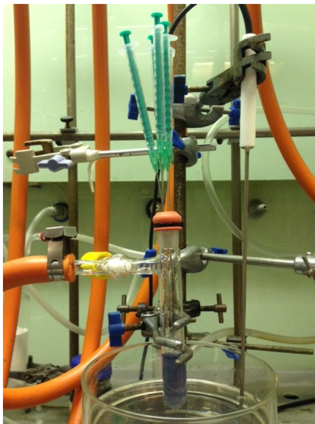
Figure S40. Experimental setup for sampling of highly air-sensitive coupling reaction
