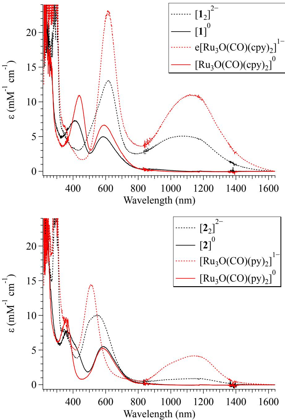
**Fig. S13.** (top) UV/vis/NIR of **1** and  $(\mathbf{1}_2)^{2-}$  in black, and  $[Ru_3O(OAc)_6(CO)(cpy)_2]$  and  $[Ru_3O(OAc)_6(CO)(cpy)_2]^-$  in red in THF at 25 °C with  $Co(cp^*)_2$  as a chemical reductant. (bottom) UV/vis/NIR of **2** and  $(\mathbf{2}_2)^{2-}$  in black, and  $[Ru_3O(OAc)_6(CO)(py)_2]$  and  $[Ru_3O(OAc)_6(CO)(py)_2]^-$  in red in THF at 25 °C with  $Co(cp^*)_2$  as a chemical reductant.
