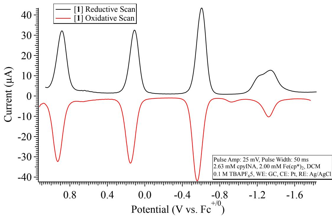
**Fig. S20.** Differential pulse voltammogram of **1** in DCM at analyte concentrations of 2.63 mM with 0.1 M  $\text{TBAPF}_6$  and an internal standard of decamethylferrocene ( $E_{1/2} = -0.58$  V vs.  $\text{Fc}^{+0}$ ). DPV's were recorded using a pulse amplitude of 25 mV, a pulse width of 50 ms and referenced to the ferrocene +/0 redox couple.
