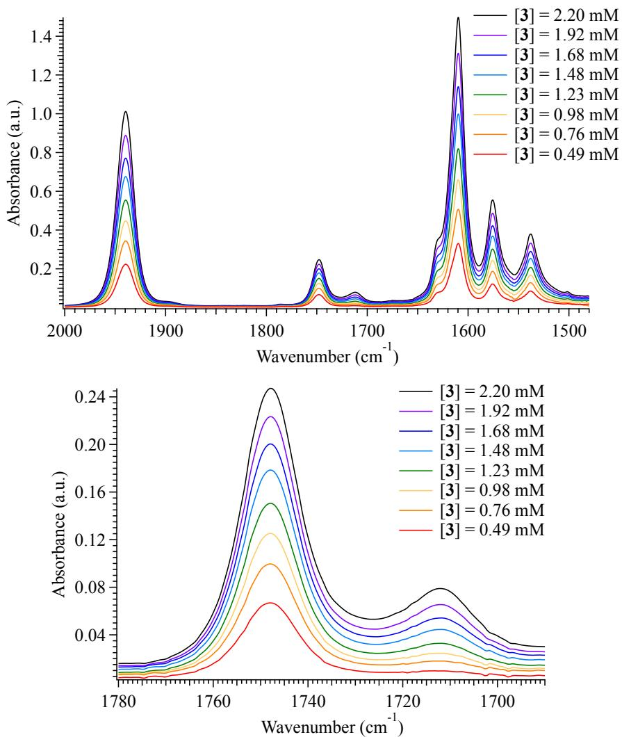
**Fig. S3.** (top) FTIR Spectrum of **3** in DCM at 25 °C. (bottom)  $\nu(\text{COOH})$  stretching region.
