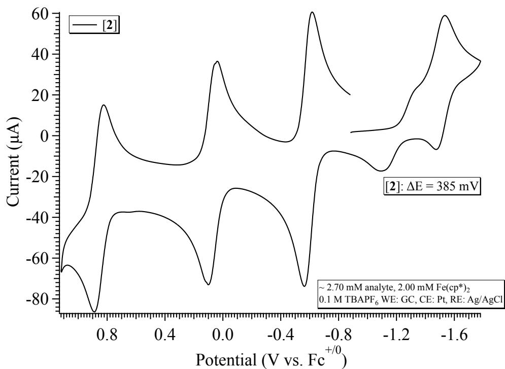
**Fig. S17.** Cyclic voltammogram of **2** in DCM at analyte concentrations of 2.70 mM with 0.1 M TBAPF<sub>6</sub> and an internal standard of decamethyl ferrocene ( $E_{1/2} = -0.58 \text{ V}$  vs.  $\text{Fc}^{+/-0}$ ). CV's were recorded at 100 mV/s and referenced to the ferrocene  $+/-0$  redox couple.
