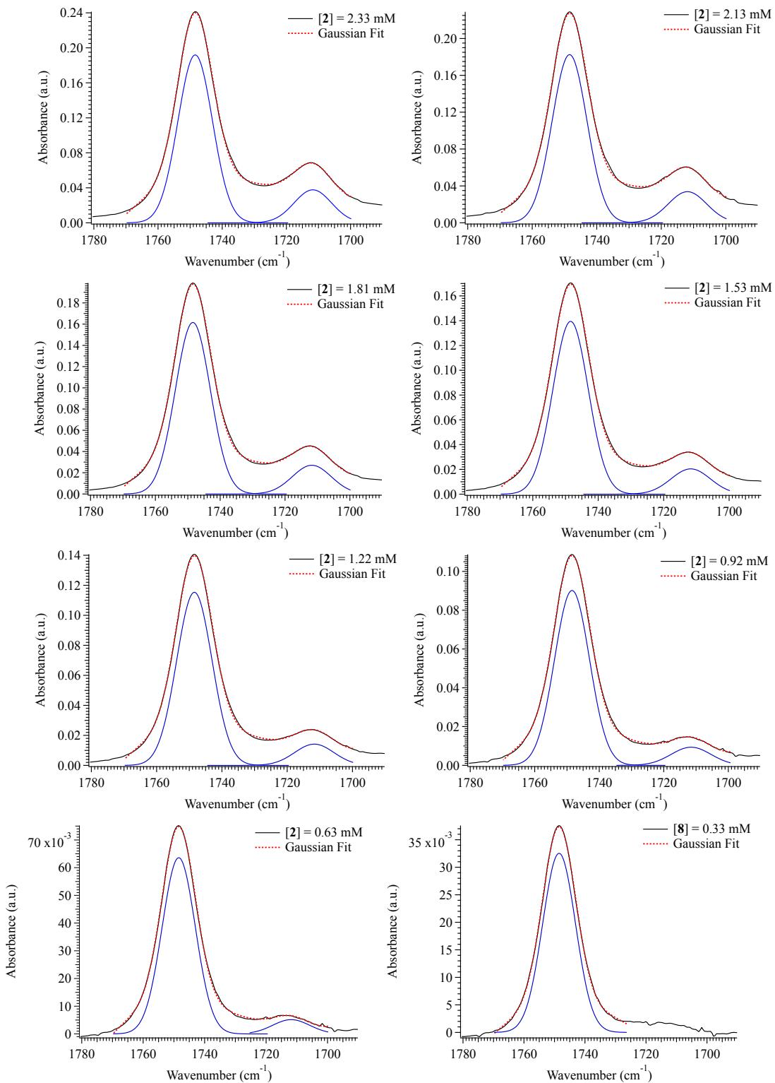
**Fig. S5.** FTIR Gaussian fits of  $\nu(\text{COOH})$  stretching region of **2** in DCM.
