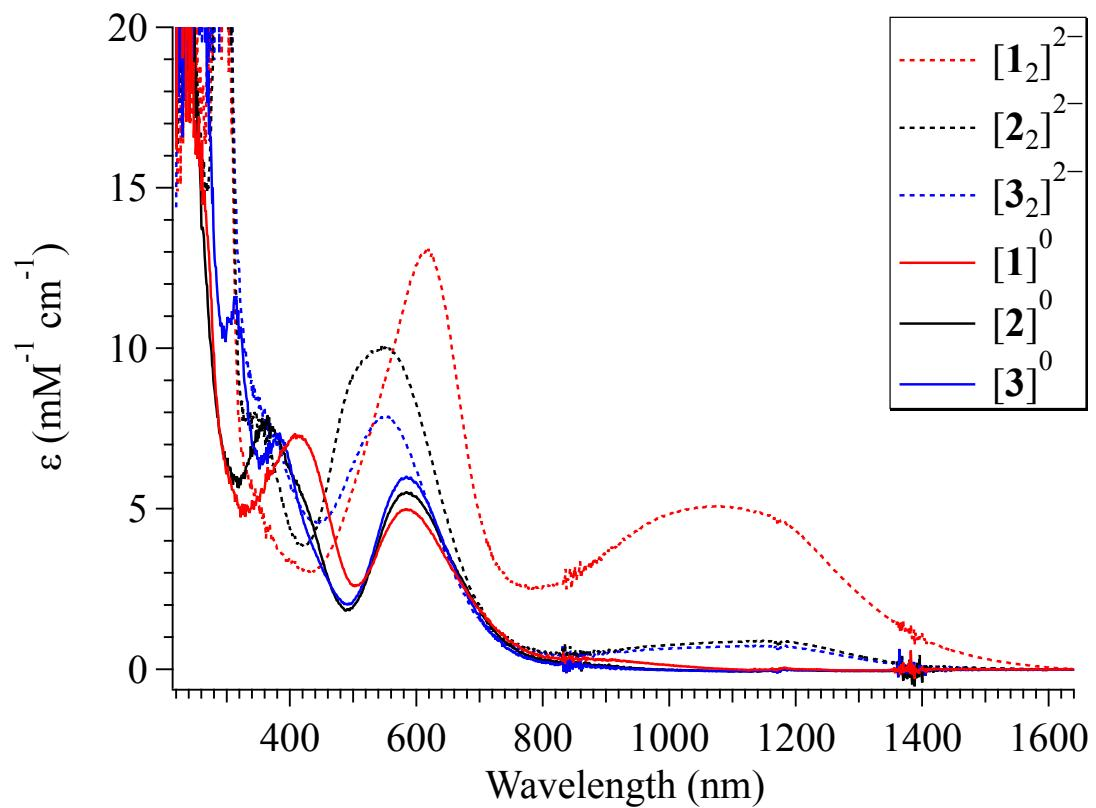
**Fig. S19.** UV/vis/NIR of **1–3** (solid) and **(1<sub>2</sub>)<sup>2-</sup>–(3<sub>2</sub>)<sup>2-</sup>** (dashed) in THF at 25 °C with Co(cp\*)<sub>2</sub> used as a chemical reductant.
