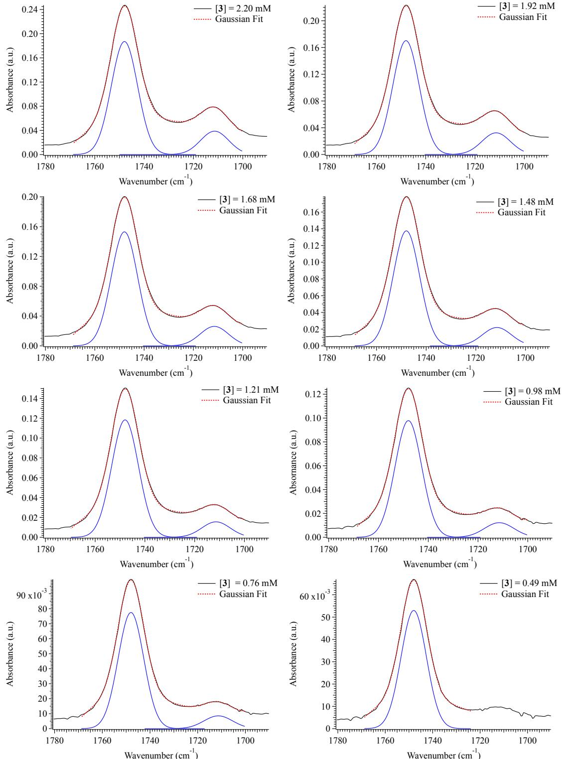
**Fig. S6.** FTIR Gaussian fits of  $\nu(\text{COOH})$  stretching region of **3** in DCM.
