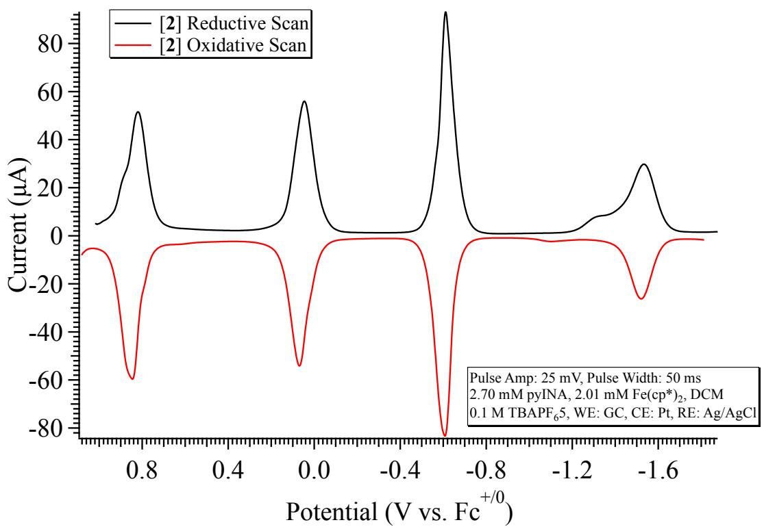
**Fig. S21.** Differential pulse voltammogram of **2** in DCM at analyte concentrations of 2.70 mM with 0.1 M TBAPF<sub>6</sub> and an internal standard of decamethyl ferrocene ( $E_{1/2} = -0.58$  V vs. Fc<sup>+/-</sup>). DPV's were recorded using a pulse amplitude of 25 mV, a pulse width of 50 ms and referenced to the ferrocene +/0 redox couple.
