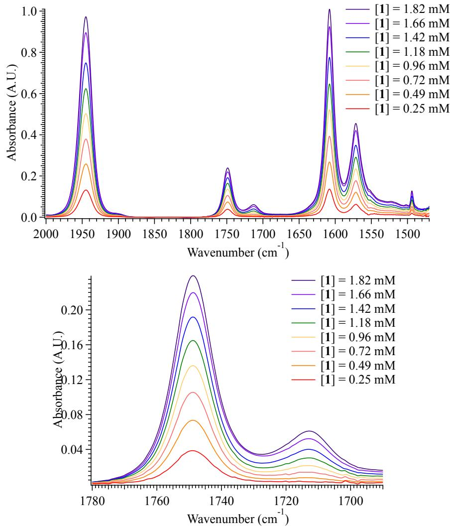
**Fig. S1.** (top) FTIR Spectrum of **1** in DCM at 25 °C. (bottom)  $\nu(\text{COOH})$  stretching region.
