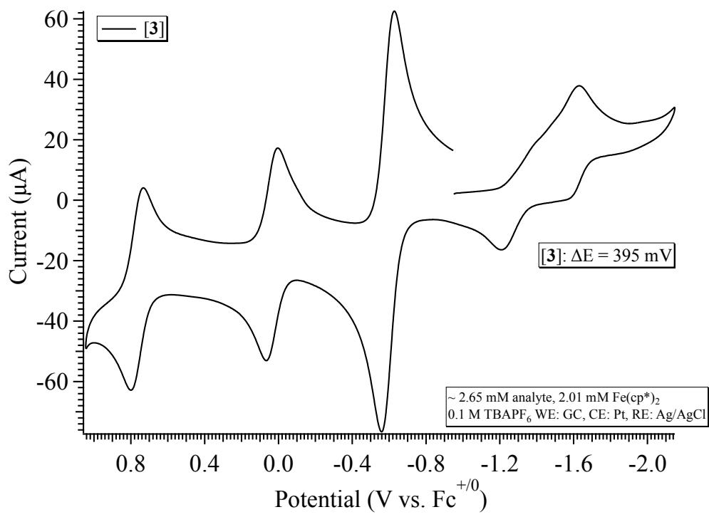
**Fig. S18.** Cyclic voltammogram of 3 in DCM at analyte concentrations of 2.65 mM with 0.1 M TBAPF<sub>6</sub> and an internal standard of decamethyl ferrocene ( $E_{1/2} = -0.58$  V vs.  $\text{Fc}^{+/-0}$ ). CV's were recorded at 100 mV/s and referenced to the ferrocene  $+/-0$  redox couple.
