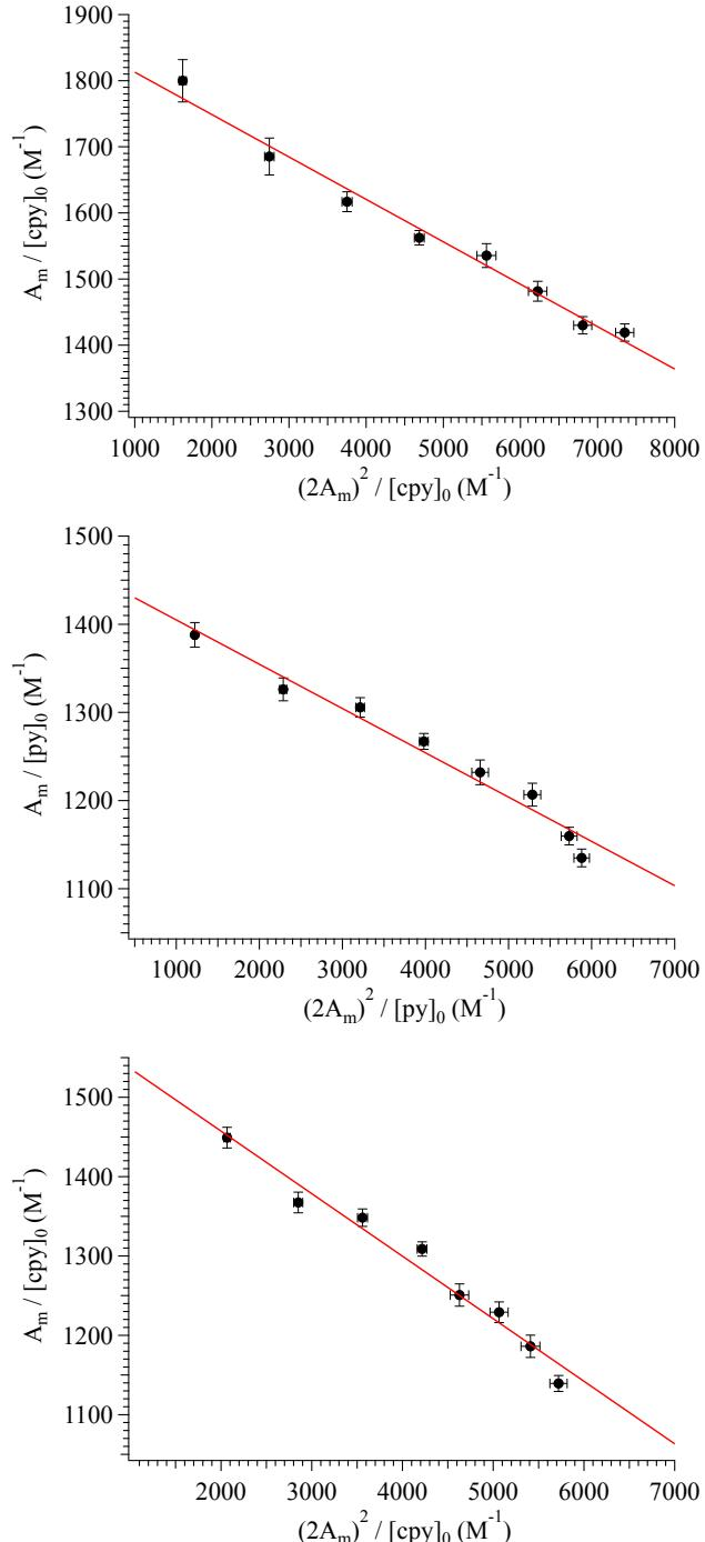
**Fig. S9.** Linear regression of integrated spectral areas for **1** (top), **2** (middle) **3** (bottom). Left side represents monomeric band while right side represents dimer band.  $[M]_0$  is the stoichiometric concentration of the solute,  $A_m$  is the integrated spectral area of the monomer band, and  $\varepsilon_m$  is the extinction coefficient of the monomer band.
