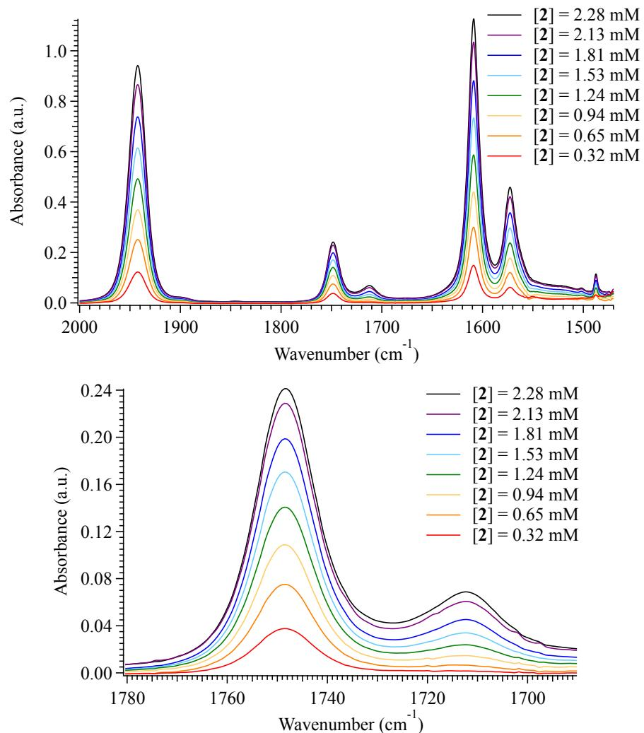
**Fig. S2.** (top) FTIR Spectrum of **2** in DCM at 25 °C. (bottom)  $\nu(\text{COOH})$  stretching region.
