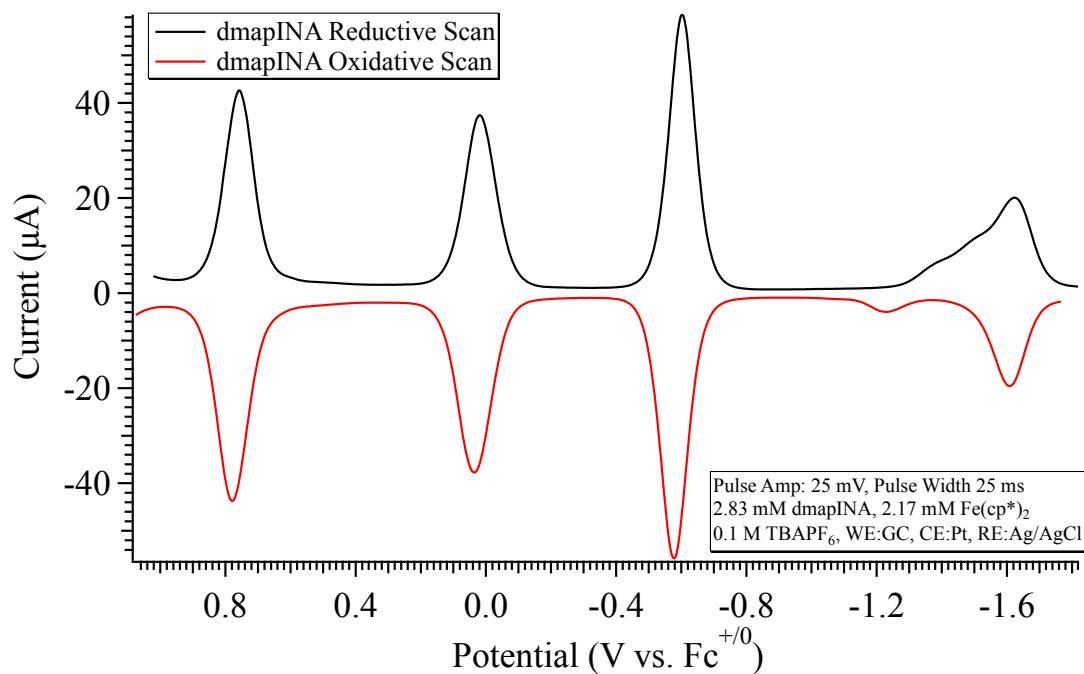
**Fig. S22.** Differential pulse voltammogram of **3** in DCM at analyte concentrations of 2.63 mM with 0.1 M  $\text{TBAPF}_6$  and an internal standard of decamethyl ferrocene ( $E_{1/2} = -0.58$  V vs.  $\text{Fc}^{+/0}$ ). DPV's were recorded using a pulse amplitude of 25 mV, a pulse width of 50 ms and referenced to the ferrocene +/0 redox couple.
