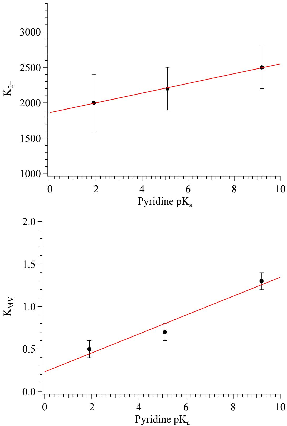
**Fig. S15.** (top) Plot of K<sub>2-</sub> vs. pyridine pK<sub>a</sub>. (bottom) Plot of K<sub>MV</sub> vs. pyridine pK<sub>a</sub>.
