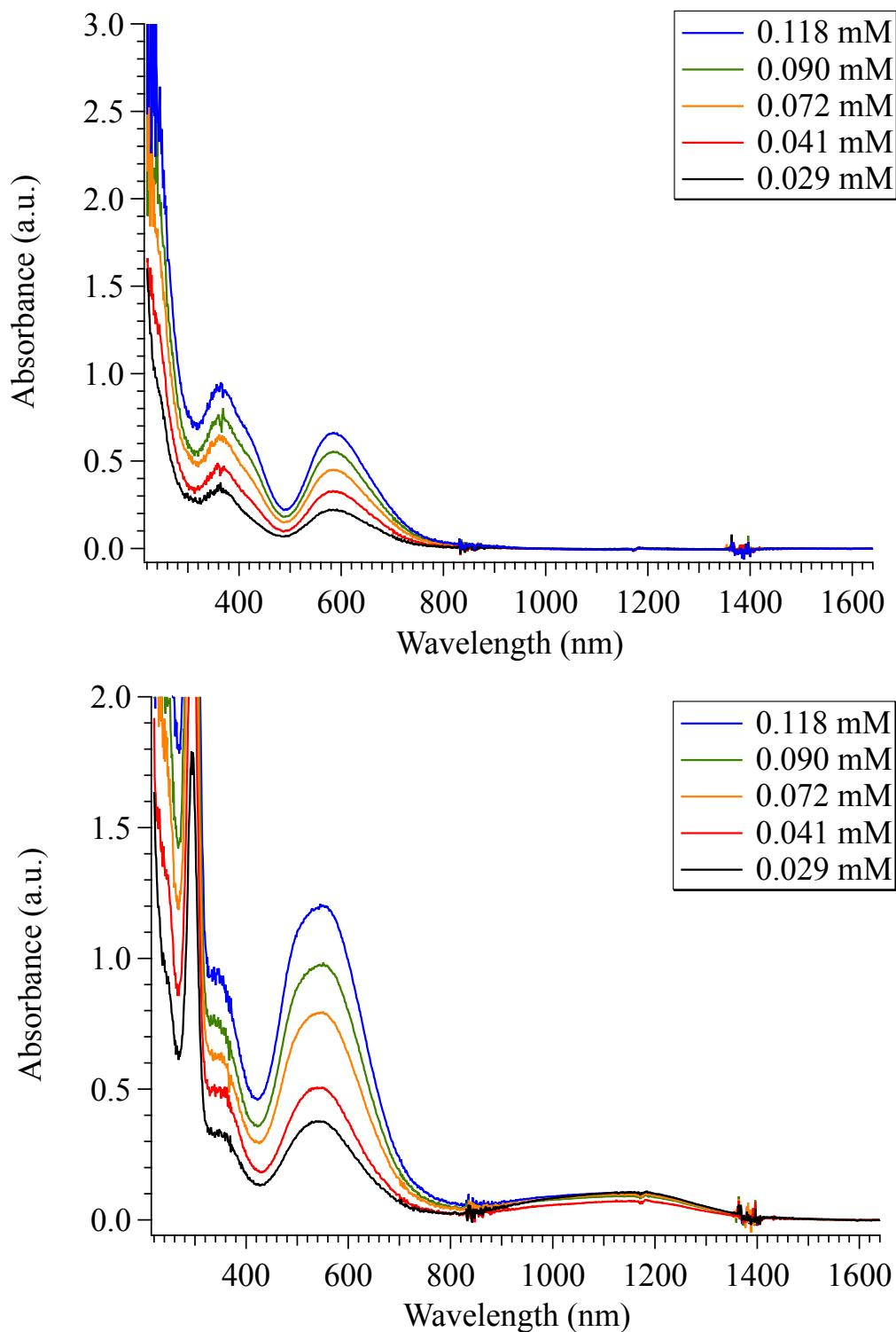
**Fig. S11.** (top) UV/vis/NIR spectra of **2** in THF. (bottom) UV/vis/NIR spectra  $(\mathbf{2}_2)^{2-}$  in THF with  $\text{Co}(\text{cp}^*)_2$  as a chemical reductant.
