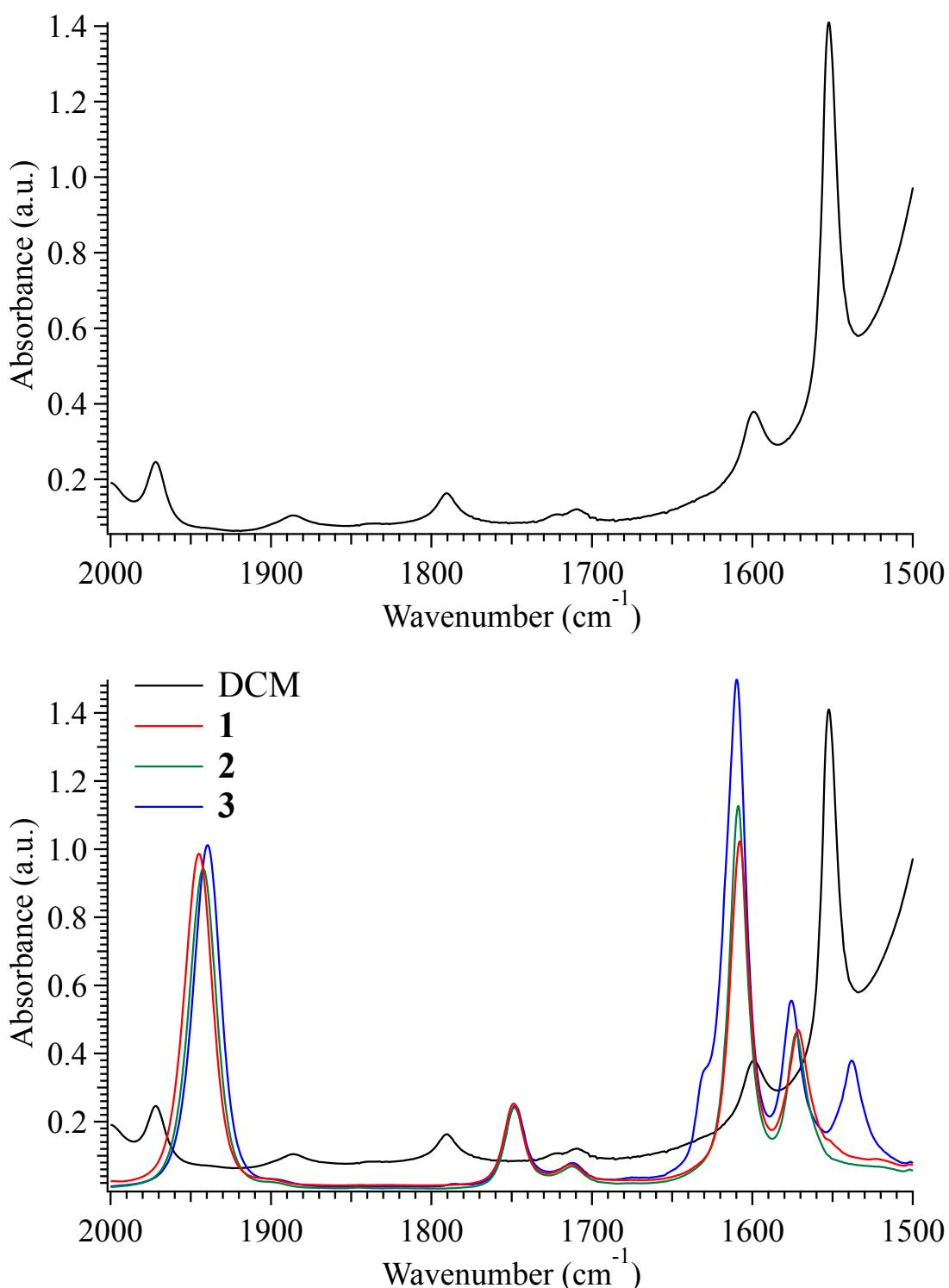
**Fig. S8.** (top) FTIR spectrum of DCM at a path length of 2.0 mm. (bottom) Overlaid FTIR spectrum of DCM and solvent subtracted **1–3**, noting the overlapping absorbance's between 1730 and 1700  $\text{cm}^{-1}$ .
