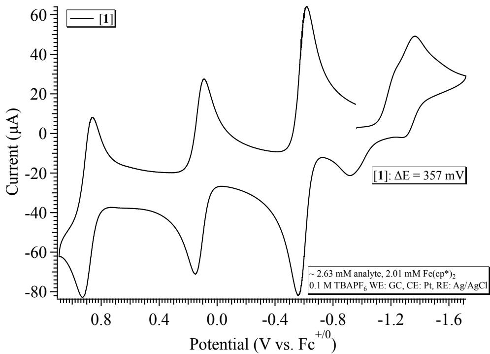
**Fig. S16.** Cyclic voltammogram of **1** in DCM at analyte concentrations of 2.63 mM with 0.1 M TBAPF<sub>6</sub> and an internal standard of decamethyl ferrocene ( $E_{1/2} = -0.58 \text{ V}$  vs.  $\text{Fc}^{+/-}$ ). CV's were recorded at 100 mV/s and referenced to the ferrocene  $+/-$  redox couple.
