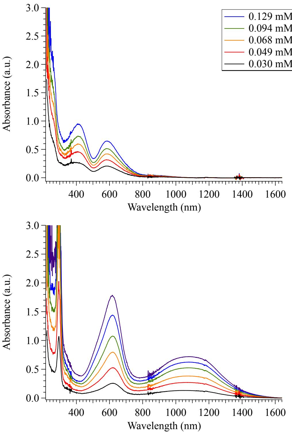
**Fig. S10.** (top) UV/vis/NIR spectra of **1** in THF. (bottom) UV/vis/NIR spectra **(1<sub>2</sub>)<sup>2-</sup>** in THF with Co(cp\*)<sub>2</sub> as a chemical reductant.
