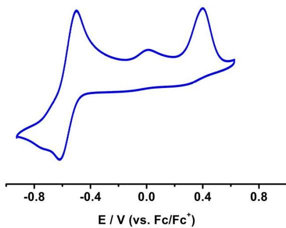
**Figure S81.** Cyclic voltammogram of **4c** in  $\text{CH}_2\text{Cl}_2/0.1 \text{ M} [\text{nBu}_4\text{N}][\text{PF}_6]$  at room temperature. Scan rate:  $100 \text{ mVs}^{-1}$ .
