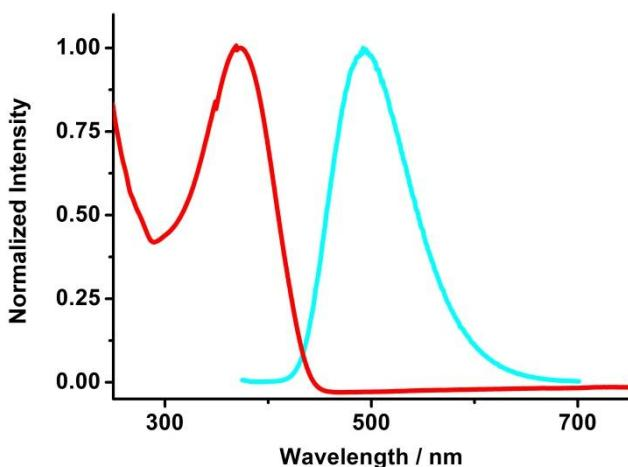
**Figure S74.** The normalized absorption (red line) and fluorescence (cyan line) spectra of **4a** in  $\text{CH}_2\text{Cl}_2$ .
