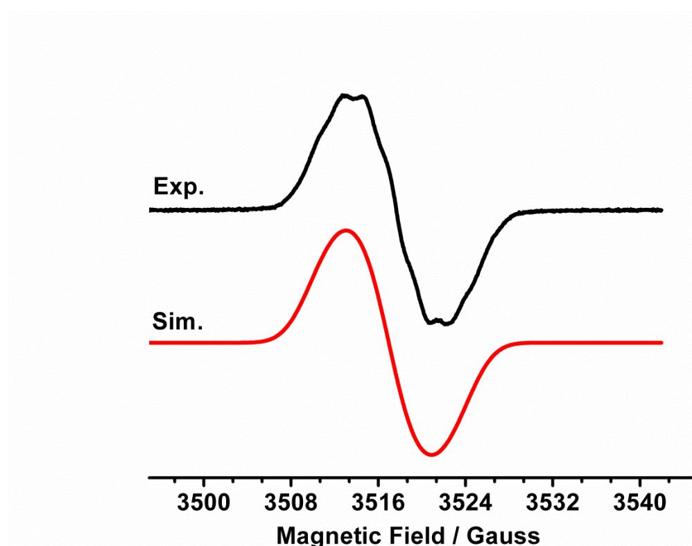
**Figure S82.** Experimental (top, black) EPR spectrum of  $[4b^{*+}] \bullet [B(C_6F_5)_4]^-$  in fluorobenzene at 298 K; simulated (bottom, red) EPR spectrum obtained using  $g = 2.0051$ ,  $a(^{11}B) = 1.77$  G,  $a(^{10}B) = 1.02$  G,  $a(^{14}N) = 0.78$  G,  $a(^1H) = 1.29$  G.
