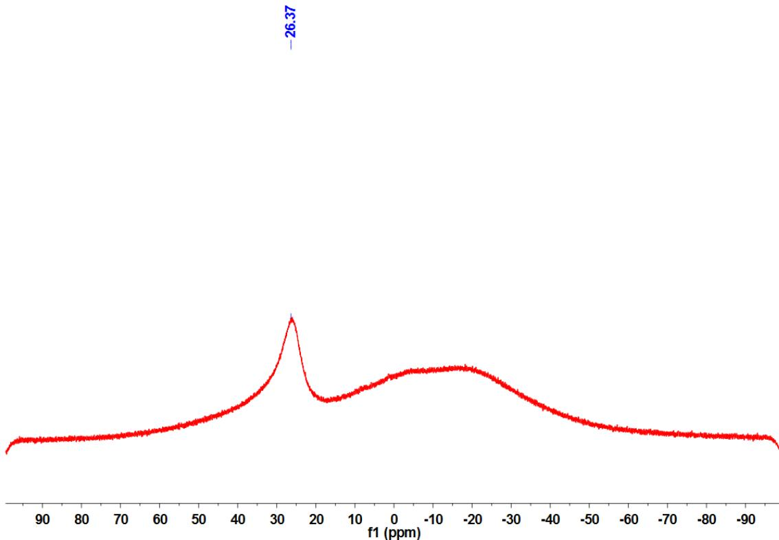
**Figure S32.** <sup>11</sup>B NMR spectrum of **4b** in  $C_6D_6$ .
