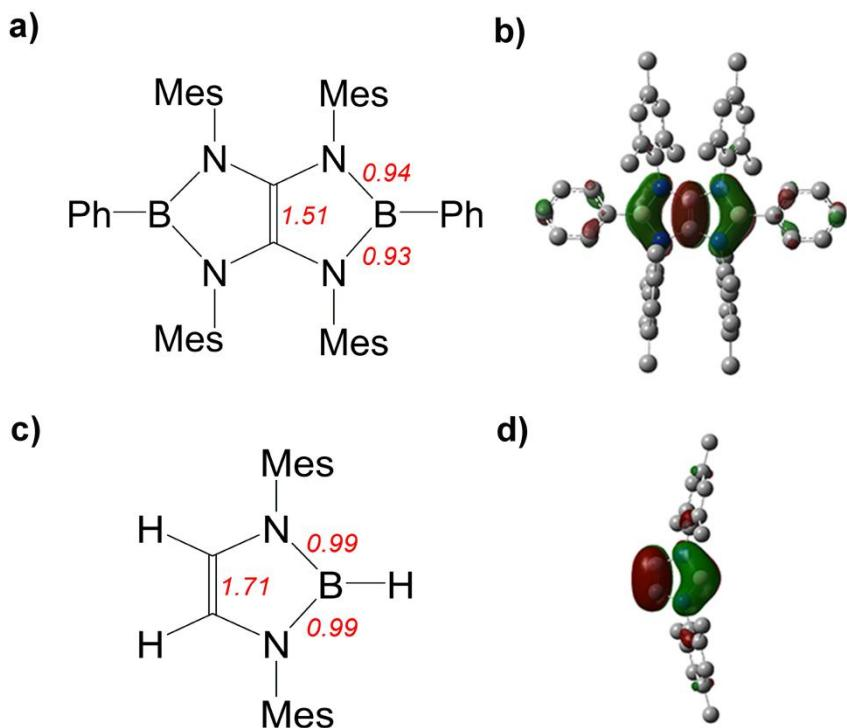
**Figure S86.** The Wiberg bond index values of **4a** (a) and 1,3-dimesityl-1,3,2-diazaborole (c) calculated at the M062X/6-31G(d,p) level. The plots of the HOMO of **4a** (b) and 1,3-dimesityl-1,3,2-diazaborole (d) (H atoms are omitted for clarity).
