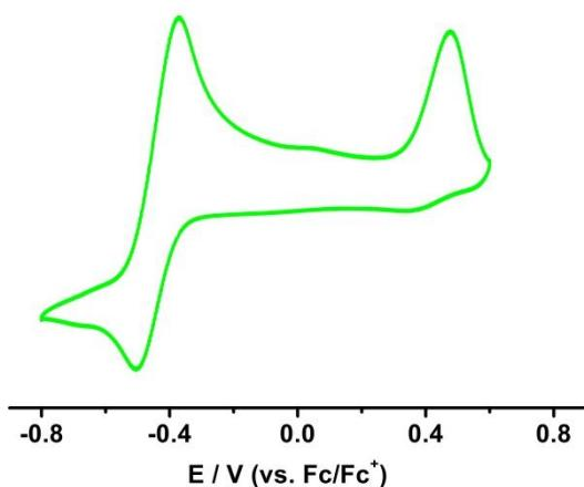
**Figure S80.** Cyclic voltammogram of **4b** in  $\text{CH}_2\text{Cl}_2/0.1 \text{ M} [\text{nBu}_4\text{N}][\text{PF}_6]$  at room temperature. Scan rate:  $100 \text{ mVs}^{-1}$ .
