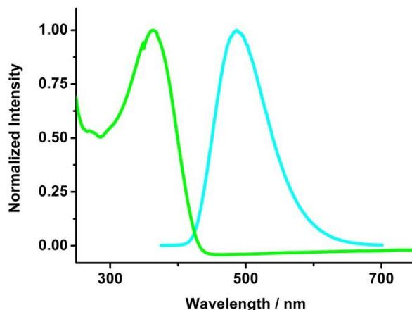
**Figure S75.** The normalized absorption (green line) and fluorescence (cyan line) spectra of **4b** in  $\text{CH}_2\text{Cl}_2$ .
