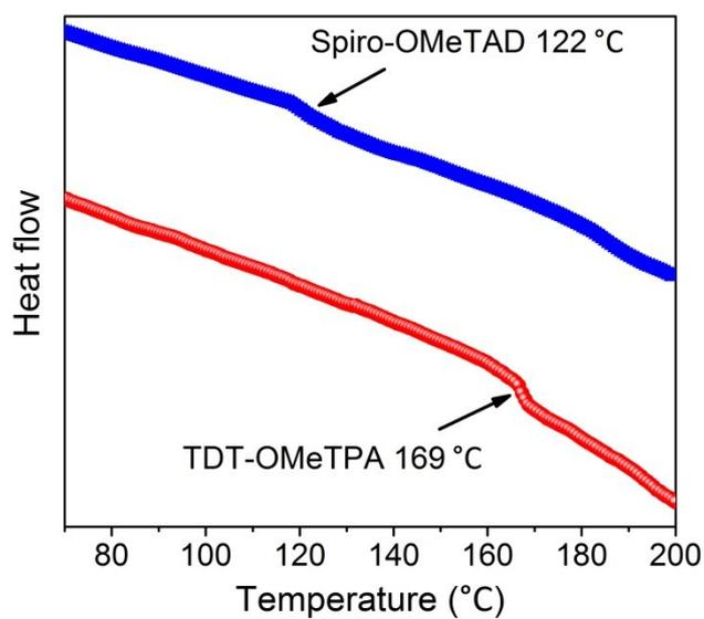
**Fig. S9.** DSC curves of TDT-OMeTPA and Spiro-OMeTAD.
