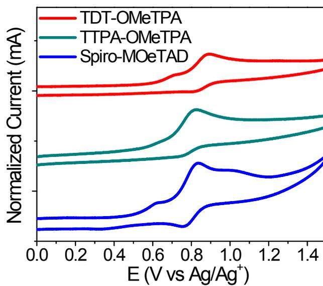
**Fig. S11.** Cyclic voltammetry (CV) curves of TDT-OMeTPA, TTPA-OMeTPA and Spiro-OMeTAD.
