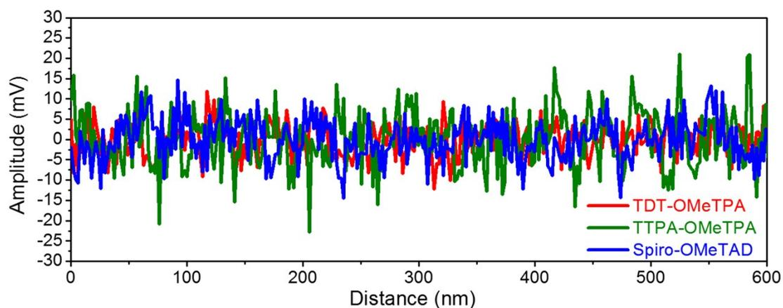
**Fig. S8.** Line profiles of AFM amplitude images for three HTM layers.
