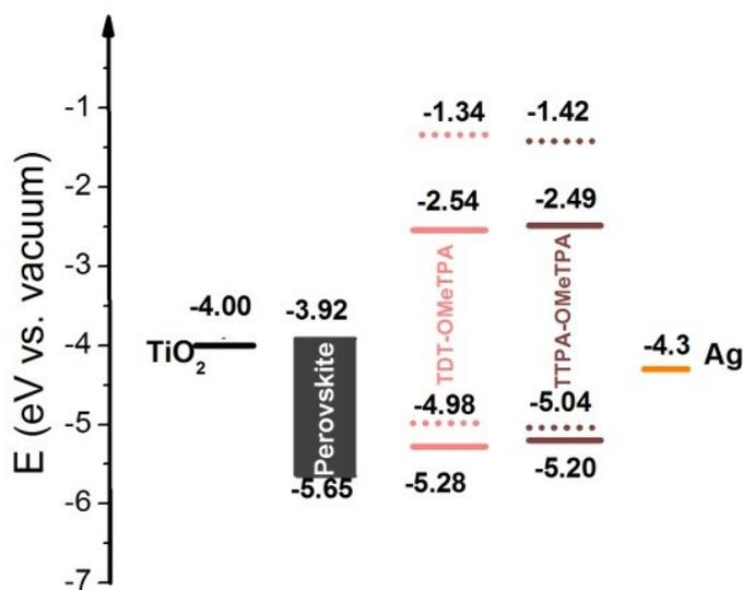
**Fig. S12.** Energy level diagram for the corresponding materials and HTMs used in TiO<sub>2</sub>/mixed-perovskite/HTM/Ag devices. Calculated HOMO and LUMO values are presented as dashed lines, experimental levels as solid lines, respectively.
