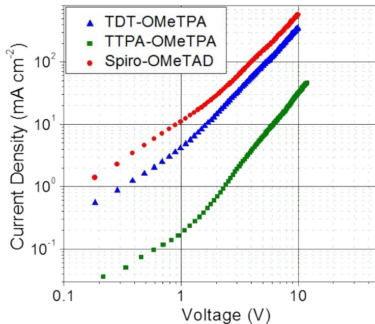
**Fig. S10.**  $J$ - $V$  characteristics of space-charge-limited current of TDT-OMeTPA, TTPA-OMeTPA and Spiro-OMeTAD.
