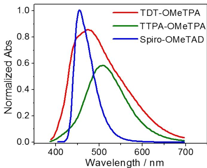
**Fig. S6.** Photo-luminance emission of TDT-OMeTPA, TTPA-OMeTPA and Spiro-OMeTAD.
