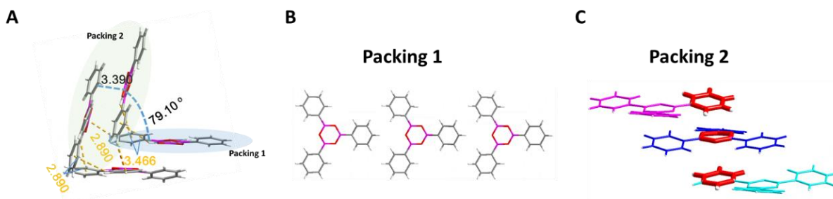
Fig. S23 Packing modes of tPBA. A: An illustration of CH... \pi interactions; B: Molecules arrangement of Packing 1; C: Molecules arrangement of Packing 2. After dehydration, the oxygen atoms are no longer exposed to the periphery of molecules and cannot build H-bonds, thus only weaker CH... \pi interactions are there to immobilize molecules. Worse, phenyl rings do not form effective \pi - \pi stacking to stabilize the excitons. The two shortcomings lead to dim RTP with short-lived lifetime.
