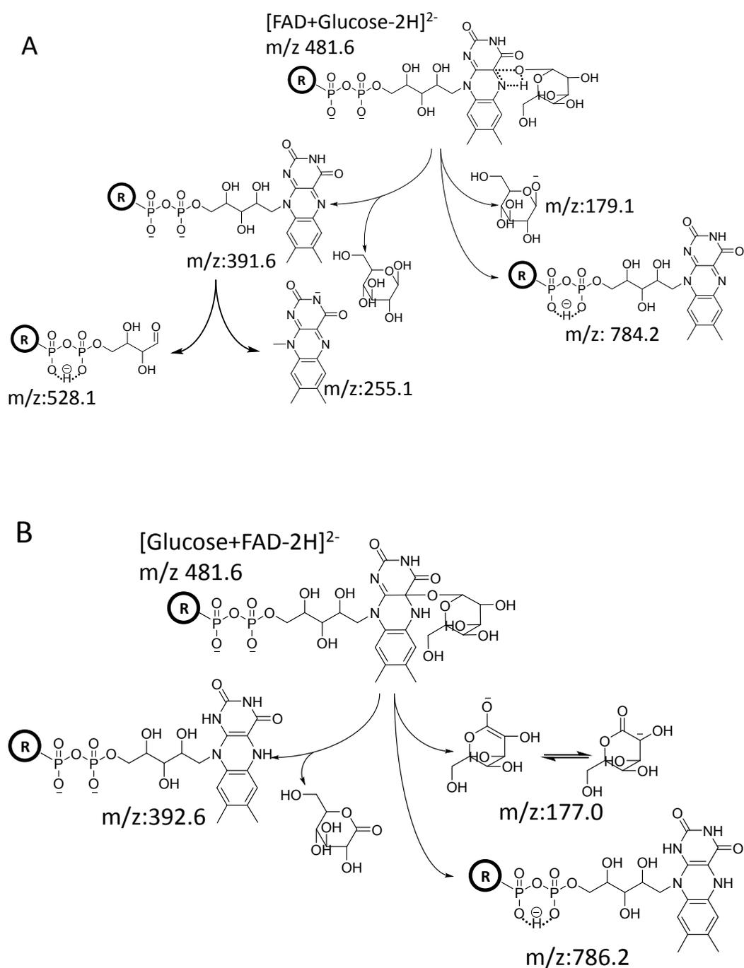
Scheme S2. Schematic diagram for fragmentation mechanism of *m/z* 481.6 generated by MS<sup>n</sup> CID in the reaction system (A) without GOx and (B) with GOx.
