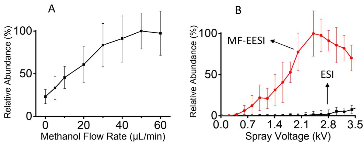
Figure S2. Optimization of MF-EESI. (A) Relative abundance of the ion of gluconic acid at  $m/z$  195.0 as a function of the methanol flow rate. (B) Comparison of signals (gluconic acid at  $m/z$  195.0) obtained by MF-EESI and ESI at different spray voltage.
