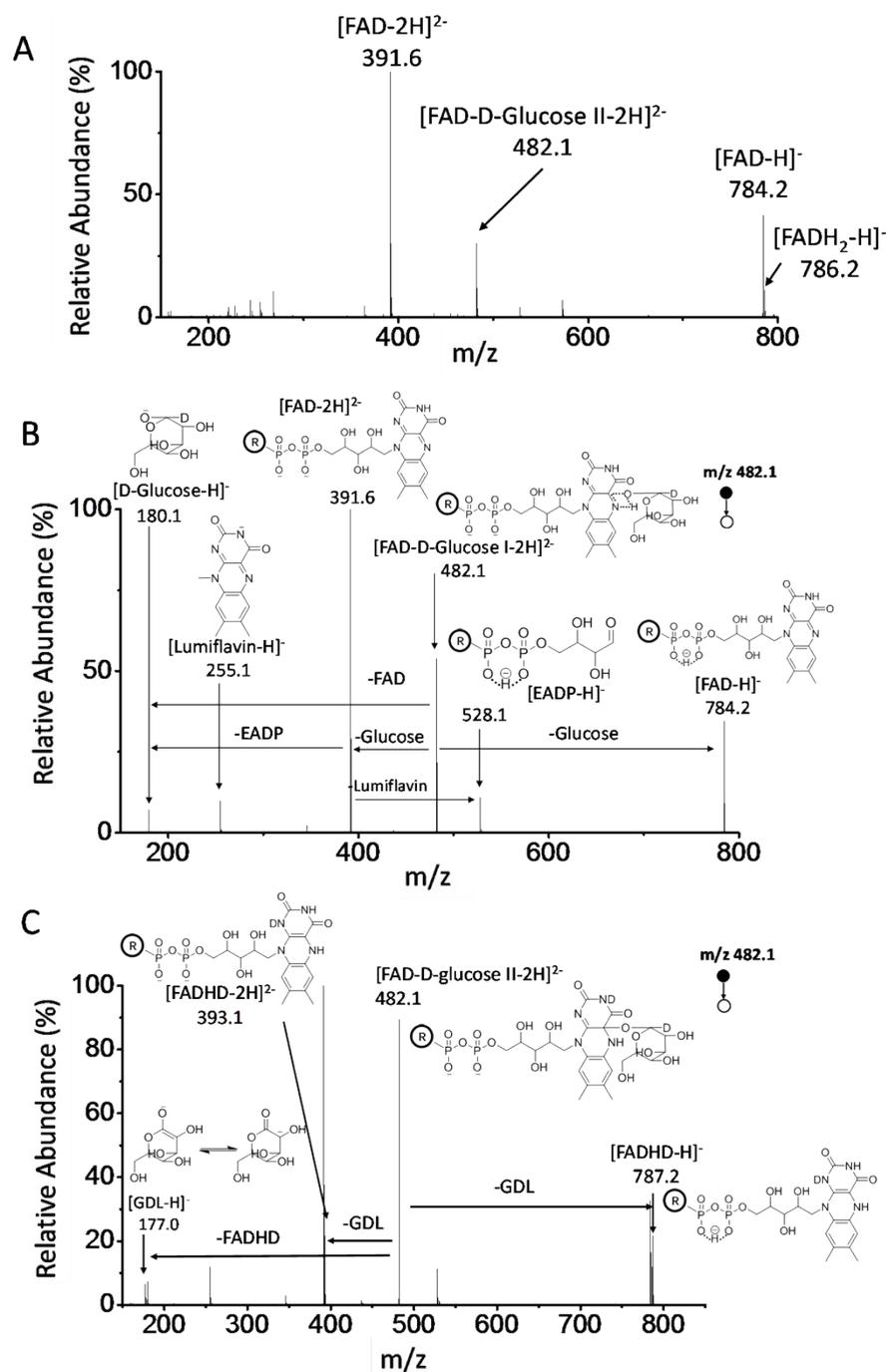
Figure S6. The isotope labeling experiment using deuterated reagent of D-glucose-1-d for the catalytic reaction. (A) Mass spectrum of the ternary mixture of D-glucose-1-d, FAD and GOx detected by MF-EESI MS. MS<sup>2</sup> CID of the two complexes of FAD and D-glucose-1-d at  $m/z$  482.1 for (B) FAD-D-Glucose I obtained from the mixture of FAD and D-glucose-1-d and (C) FAD-D-Glucose II obtained from the mixture of FAD, D-glucose-1-d and GOx.
