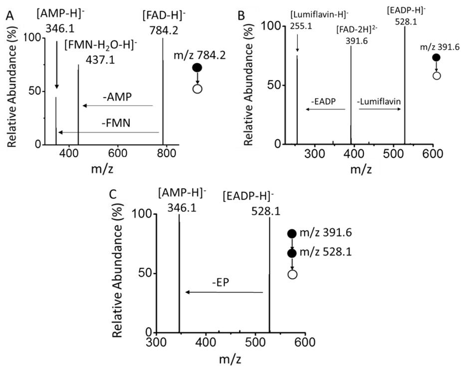
Figure S3. Structural confirmation of the FAD-Glucose I complex from the mixture of FAD and glucose by CID. (A) MS<sup>2</sup> CID of the ion at m/z 784.2. (B) MS<sup>2</sup> CID of the ion at m/z 391.6. (C) MS<sup>3</sup> CID of m/z 528.1.
