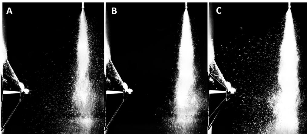
Figure S1. Actual pictures of introduction of ions from different sprays into the MS inlet. (A) Extracted sample. (B)  $50 \mu\text{L}\cdot\text{min}^{-1}$  methanol, (C) extracted sample with  $50 \mu\text{L}\cdot\text{min}^{-1}$  methanol.
