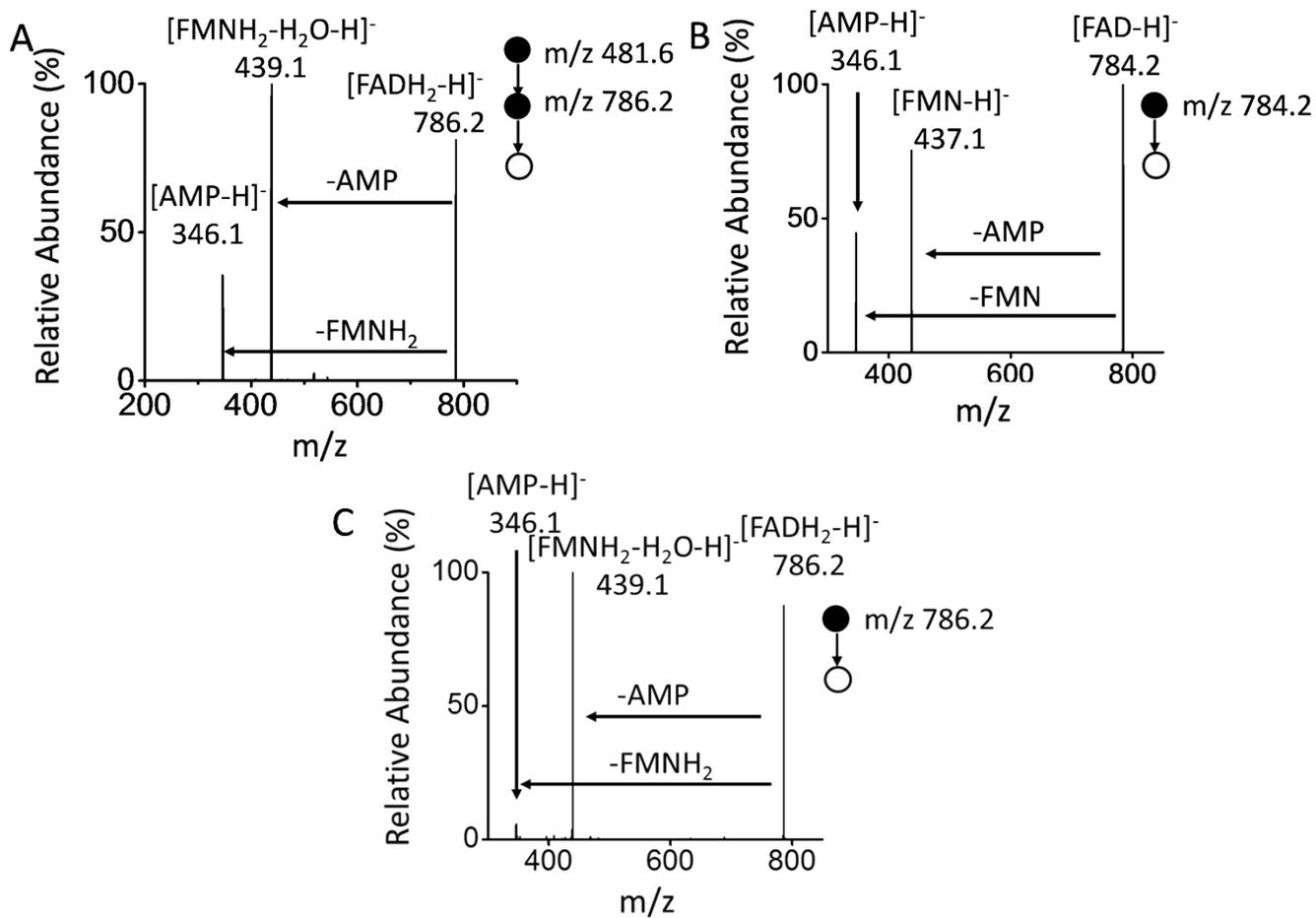
Figure S4. Structure confirmation by CID for the FAD-Glucose II complex from the mixture of FAD and glucose in the presence of GOx. (A) MS<sup>3</sup> CID of  $m/z$  481.6; (B) MS<sup>2</sup> CID of the ion at  $m/z$  784.2; (C) MS<sup>2</sup> CID of the ion at  $m/z$  786.2.
