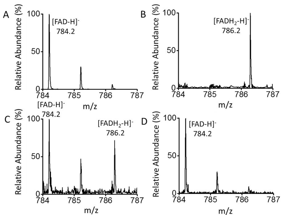
Figure S7. Mass spectra confirmation for cyclic conversion of FAD. (A) the mixture of FAD and glucose, (B) addition of GOx into the system, (C) introduction of  $O_2$  into the catalytic oxidation system, and (D) after introduction of  $O_2$ .
