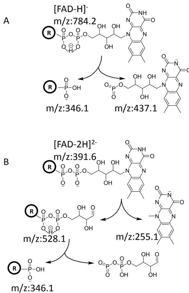
Scheme S1. The fragmentation mechanism of (A) [FAD-H]<sup>-</sup> at *m/z* 784.2 and (B) [FAD-2H]<sup>2-</sup> at *m/z* 391.6 generated by MS<sup>n</sup> CID.
