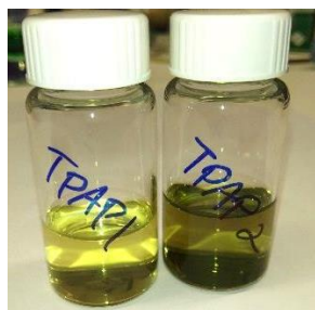
Figure S8. 1.8 mg of n\text{-Pr}_4\text{N}[\text{RuO}_4] in MeCN (10 mL). Left – synthesised; Right – commercial.
