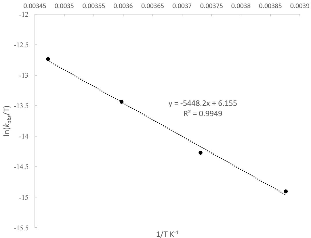
$$\Delta H^\ddagger = 10.8 \text{ kcal mol}^{-1}, \Delta S^\ddagger = -35.0 \text{ cal K}^{-1} \text{ mol}^{-1}, \Delta G^\ddagger_{298K} = 21.3 \text{ kcal mol}^{-1}$$
