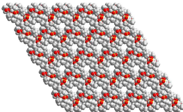
Crystal packing structure of **6g-ester** (5x5 unit cells) showing the void channels.
