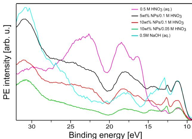
**Figure SI-3** Photoelectron spectra at resonance *a* (532.2 eV) for the same three  $\alpha$ -Fe<sub>2</sub>O<sub>3</sub> NPs aqueous solutions considered in Figure SI-2. In addition, spectra from 0.5 M HNO<sub>3</sub> and 0.5 M NaOH (measured at near *a*) aqueous solution, are shown. Unlike in Figure 4 of the manuscript spectra are shown as measured without the off-resonant photoelectron spectrum subtracted. Otherwise Figure SI-3 and Figure 4 are identical.
