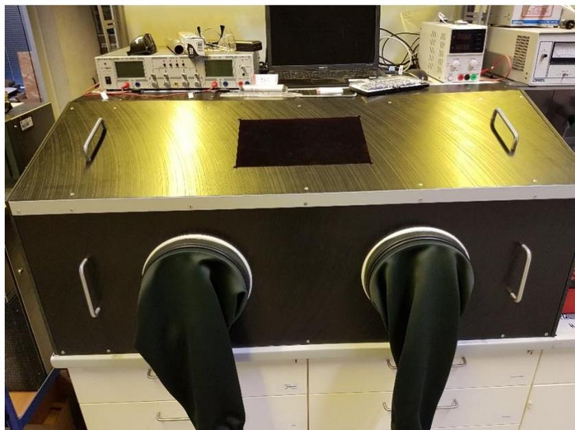
**Figure S25:** Black box with a red window used for the actinometry and quantum yield experiments.
