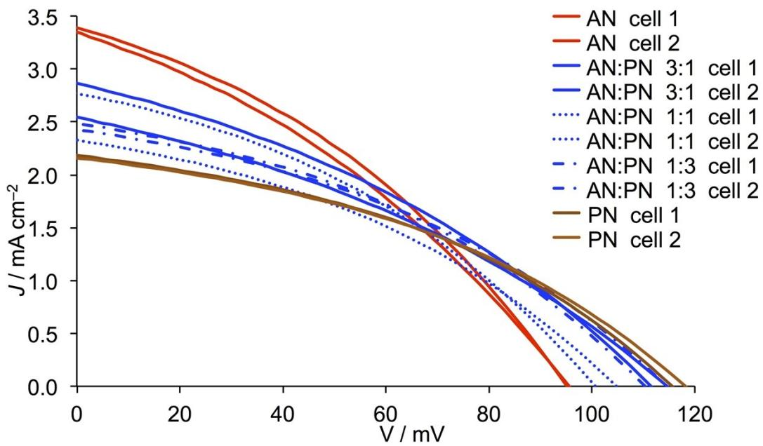
**Fig. S1.**  $J$ - $V$  curves for duplicate DSCs containing in-house screen-printed (Solaronix paste) FTO/NiO electrodes functionalized with  $[\text{Ru}(\text{bpy})_2(\text{H1})]$  and electrolytes comprising  $\text{I}_3^-/\text{I}^-$  in AN, PN or AN:PN mixed solvent. Ratios of solvents are by volume.
