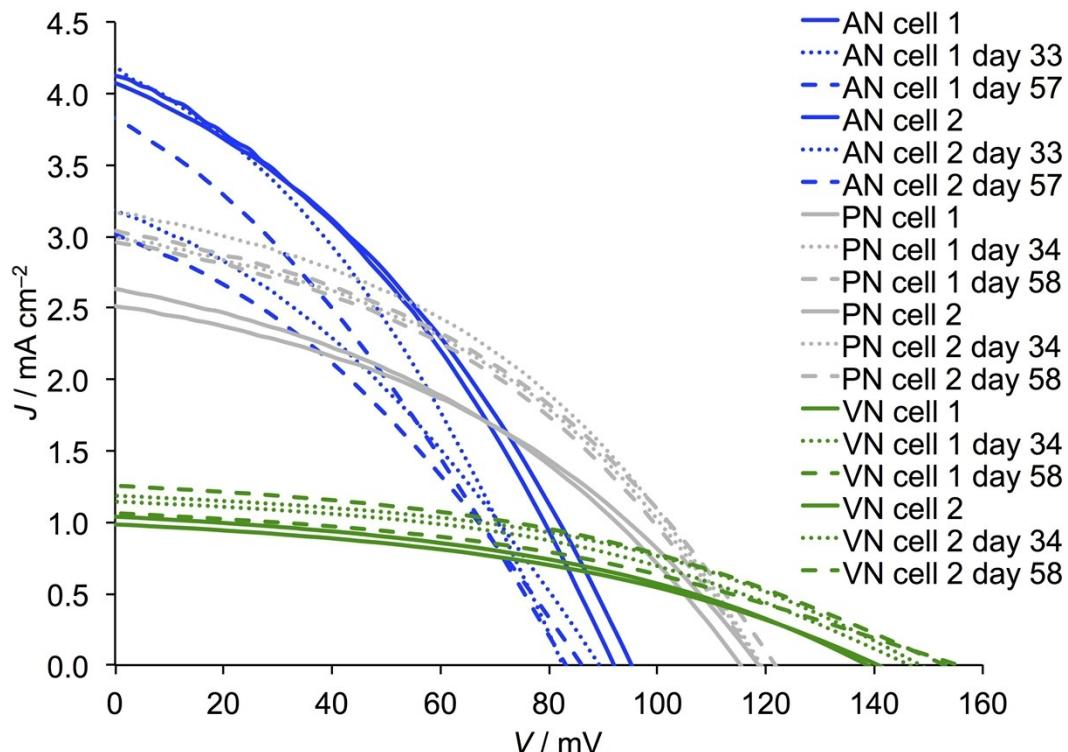
**Fig. S4.**  $J$ - $V$  curves for duplicate DSCs containing commercial FTO/NiO electrodes functionalized with  $[\text{Ru}(\text{bpy})_2(\text{H1})]$  and electrolytes comprising  $\text{I}_3^-/\text{I}^-$  in AN, PN or VN. Measurements were made on day 0, then 33 or 34, then 57 or 58 days later. Curves for MPN are omitted for clarity (see Fig. 6).
