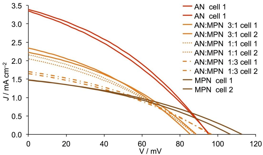
**Fig. S3.**  $J$ - $V$  curves for duplicate DSCs containing in-house screen-printed (Solaronix paste) FTO/NiO electrodes functionalized with  $[\text{Ru}(\text{bpy})_2(\text{H1})]$  and electrolytes comprising  $\text{I}_3^-/\text{I}^-$  in AN, MPN or AN:MPN mixed solvent. Ratios of solvents are by volume.
