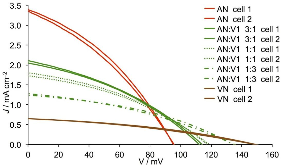
**Fig. S2.**  $J$ - $V$  curves for duplicate DSCs containing in-house screen-printed (Solaronix paste) FTO/NiO electrodes functionalized with  $[\text{Ru}(\text{bpy})_2(\text{H1})]$  and electrolytes comprising  $\text{I}_3^-/\text{I}^-$  in AN, VN or AN:VN mixed solvent. Ratios of solvents are by volume.
