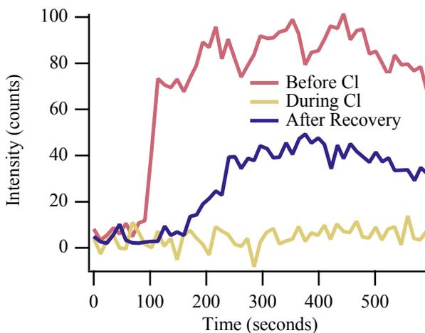
Figure S1: Recovery of the carbon “G” peak after recovery of a fuel cell poisoned by chlorine at 650 °C.
