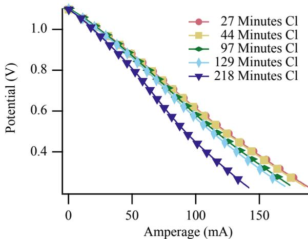
Figure S4: Hydrogen LSV of a cell operating at 700 °C.
