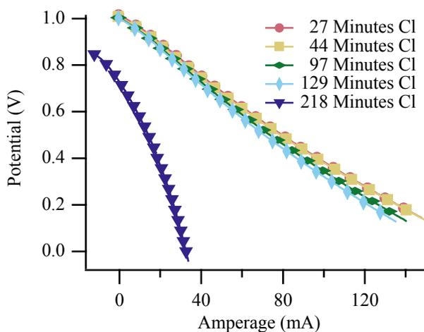
Figure S5: Biogas LSV of a cell operating at 700 °C.
