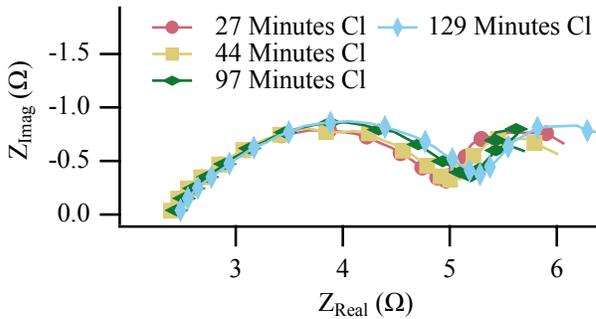
Figure S3: Biogas EIS spectra of cell operating at 700 °C.
