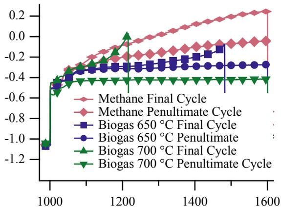
Figure S8: Failure methods for biogas at 650 °C and 700 °C (blue and green respectively) and methane at 650 °C (red). Each set shows the penultimate and final cycle for each experiment.
