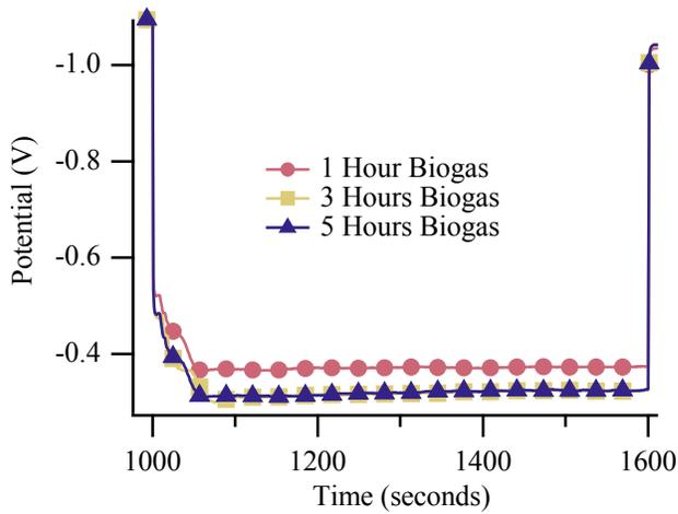
Figure S7: Potential vs. Time plots for a control biogas cycling experiment at 650 °C.
