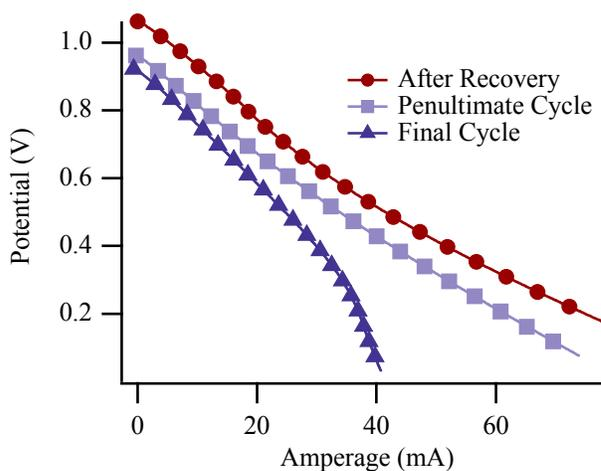
Figure S6: Performance data recovery for a cell operating at 650 °C and recovered for 1 hour in 18 sccm of H<sub>2</sub> with 55 sccm Ar carrier gas after chlorine induced failure. Blue traces above are the final two cycles of chlorine exposure.
