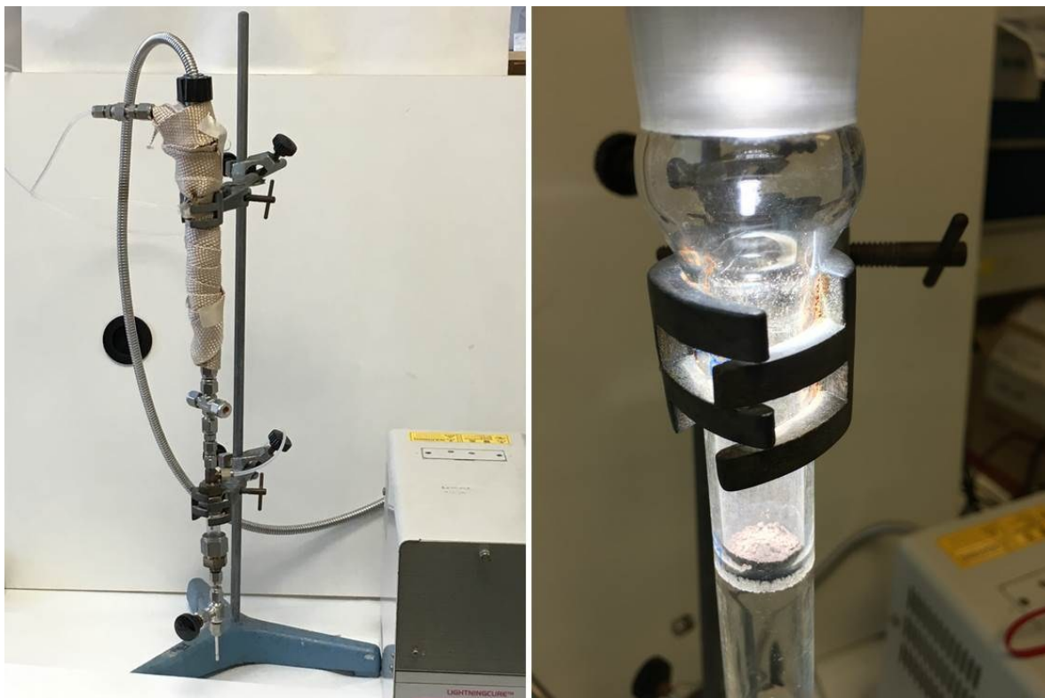
Figure S13. Digital images of the cylindrical reactor coated with the heating mantle and the optic fibre (left) and the photocatalyst loaded in the reactor with the lamp on (right).
