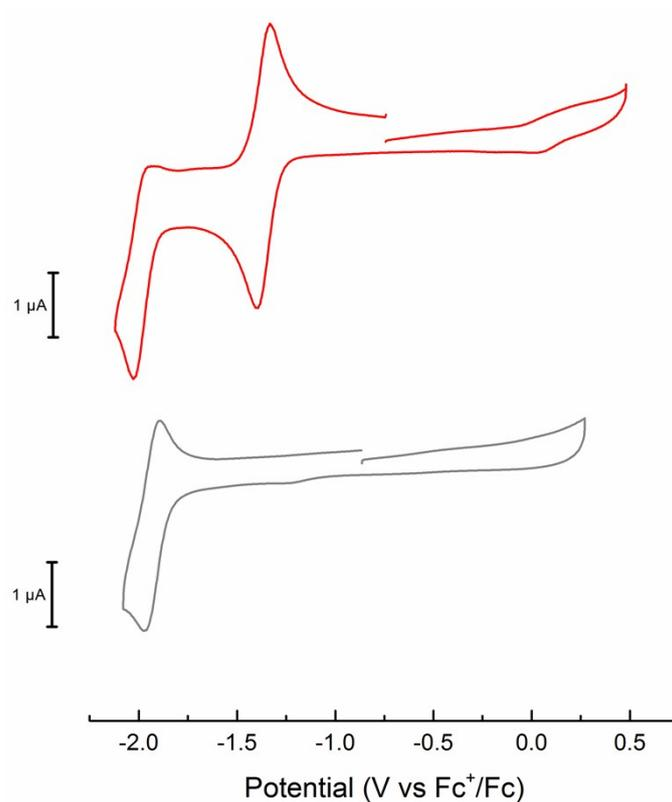
**Figure S1.** Cyclic voltammograms of  $\mathbf{1}(\text{BF}_4)_2$  (red line) and of the corresponding zinc complex (grey line) recorded in DMF (containing 0.1 M  $(n\text{-Bu})_4\text{N}(\text{BF}_4)$  as supporting electrolyte).
