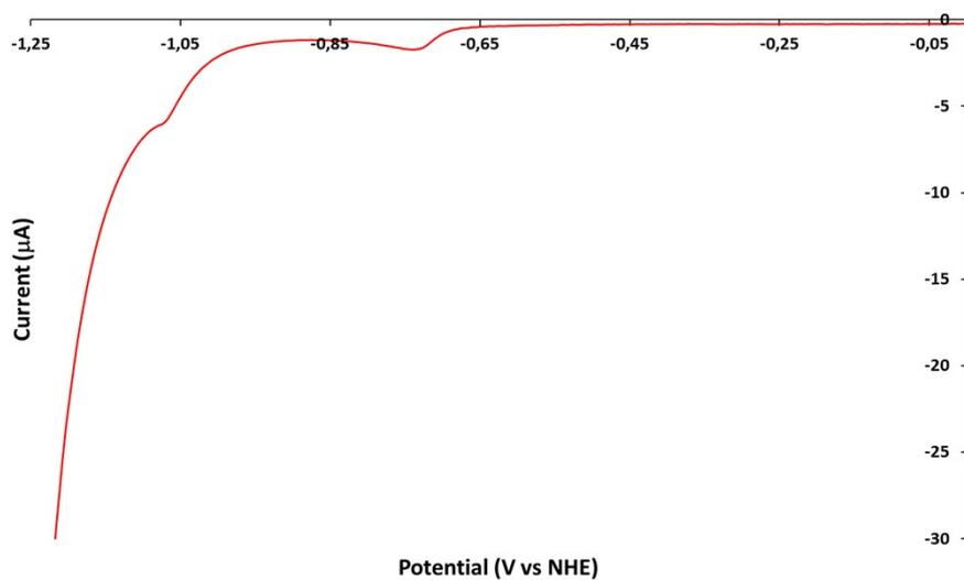
**Figure S2.** Linear sweep voltammogram of  $\mathbf{1}(\text{BF}_4)_2$  (1 mM) recorded in Tris-HCl buffer (0.1 M, pH 7) at a scan rate of  $10 \text{ mV}\cdot\text{s}^{-1}$ . Contribution from direct proton reduction at the electrode surface is observed below  $-1.2 \text{ V}$  vs NHE.
