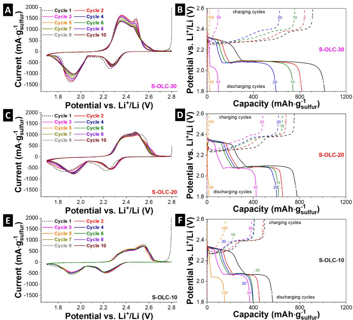
**Figure S5:** Cyclic voltammograms (measured in 3-electrode set-up) at a rate of  $0.1 \text{ mV s}^{-1}$  and galvanostatic charge/discharge (measured in 2-electrode set-up) profiles at  $336 \text{ mA g}^{-1}$  ( $0.2 \text{ C}$ ) for charging and  $168 \text{ mA g}^{-1}$  ( $0.1 \text{ C}$ ) for discharging in the potential window of  $+1.8 \text{ V}$  to  $+2.6 \text{ V}$  vs.  $\text{Li}^+/\text{Li}$  of (A and B) S-OLC-30, (C and D) S-OLC-20, and (E and F) S-OLC-10.
