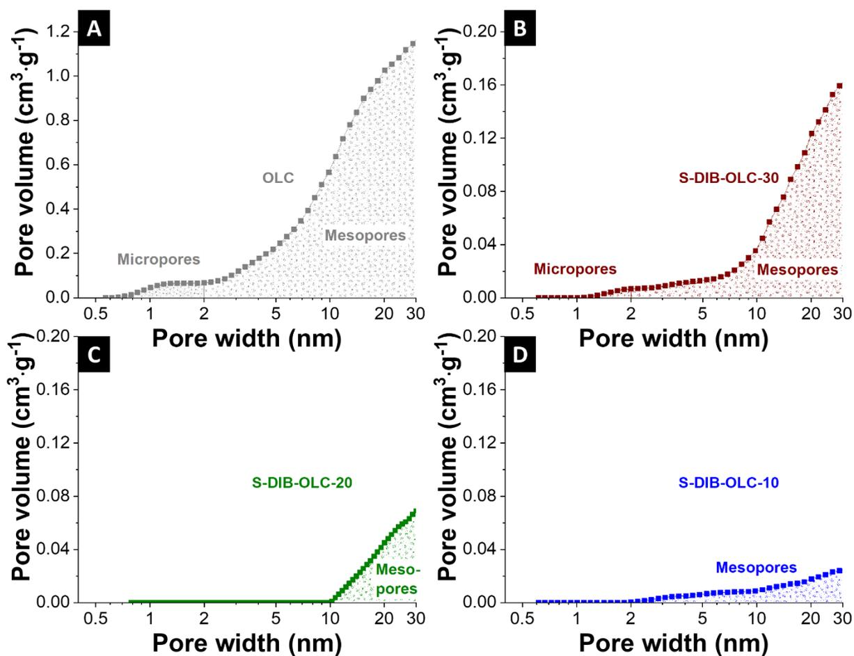
**Figure S2:** Cumulative pore size distributions per volume of carbon onions (dry powder) and S-DIB-OLC hybrids calculated with quenched-solid density functional theory from nitrogen gas sorption isotherms recorded at  $-196^\circ\text{C}$ .
