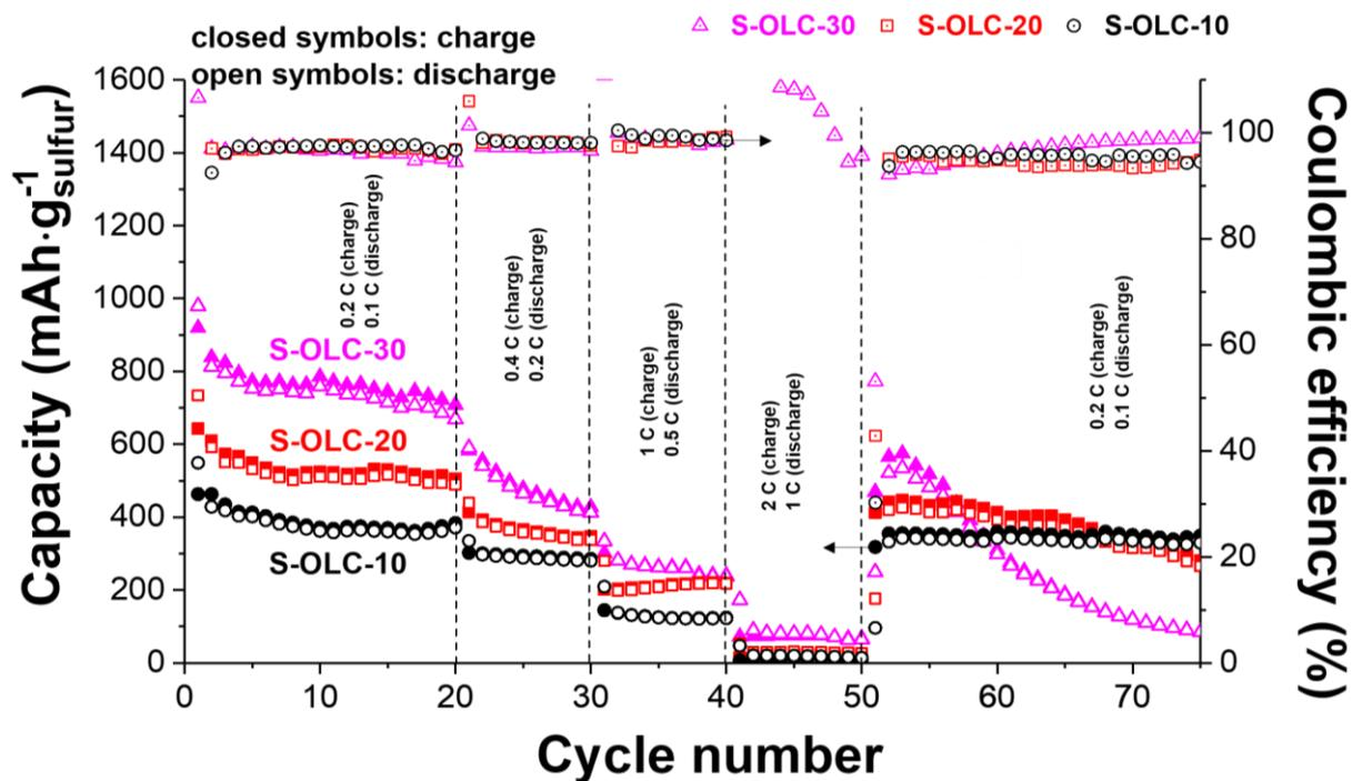
**Figure S6:** Rate handling of carbon onion / sulfur hybrids prepared by melt-diffusion measured in 3-electrode set-up.
