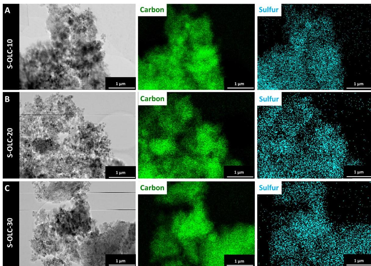
**Figure S3:** TEM micrographs of carbon onion / sulfur copolymer hybrids and their corresponding elemental EDX mappings.
