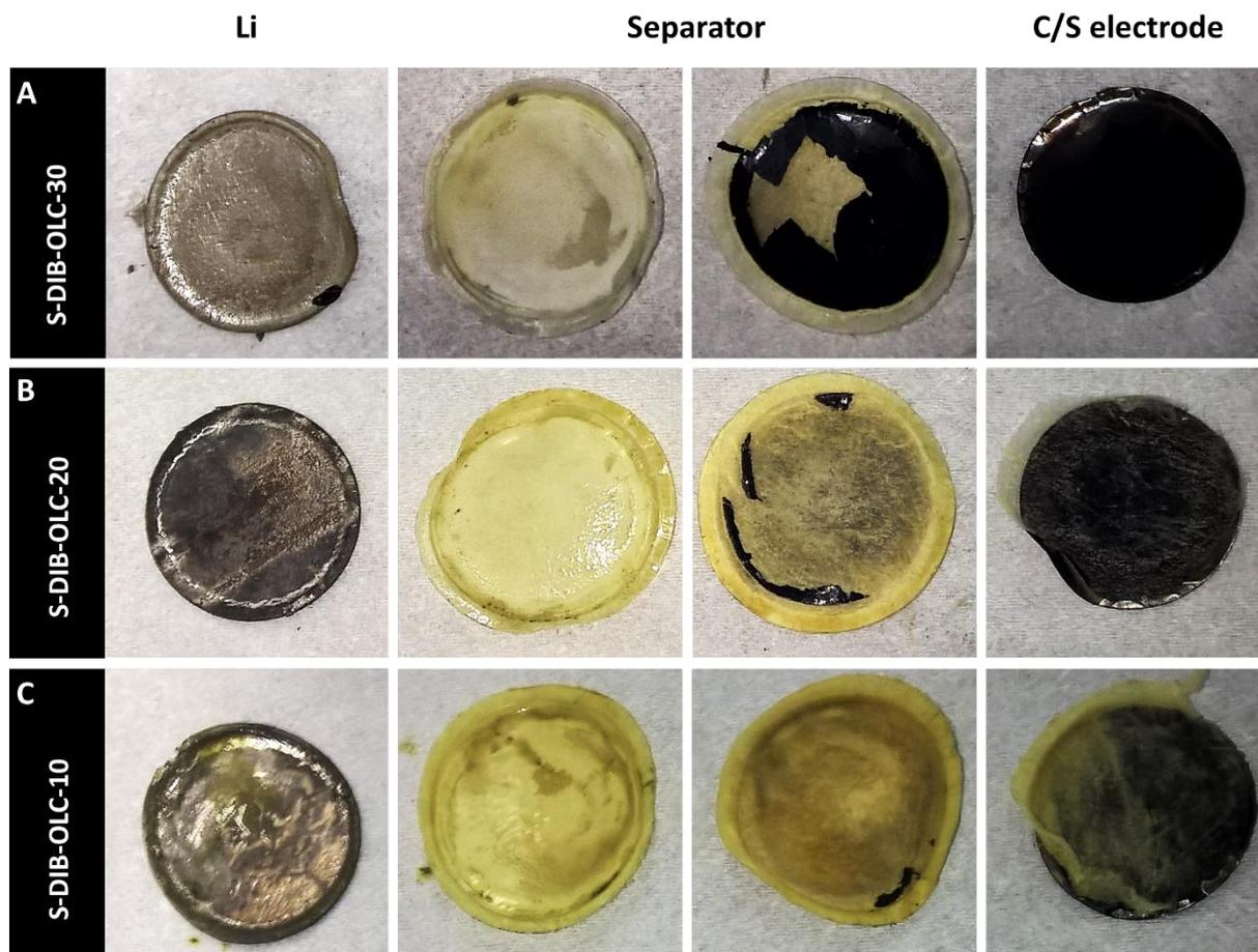
**Figure S7:** Digital photographs of carbon onion / sulfur copolymer hybrid cell parts after 100 charge-discharge cycles.
