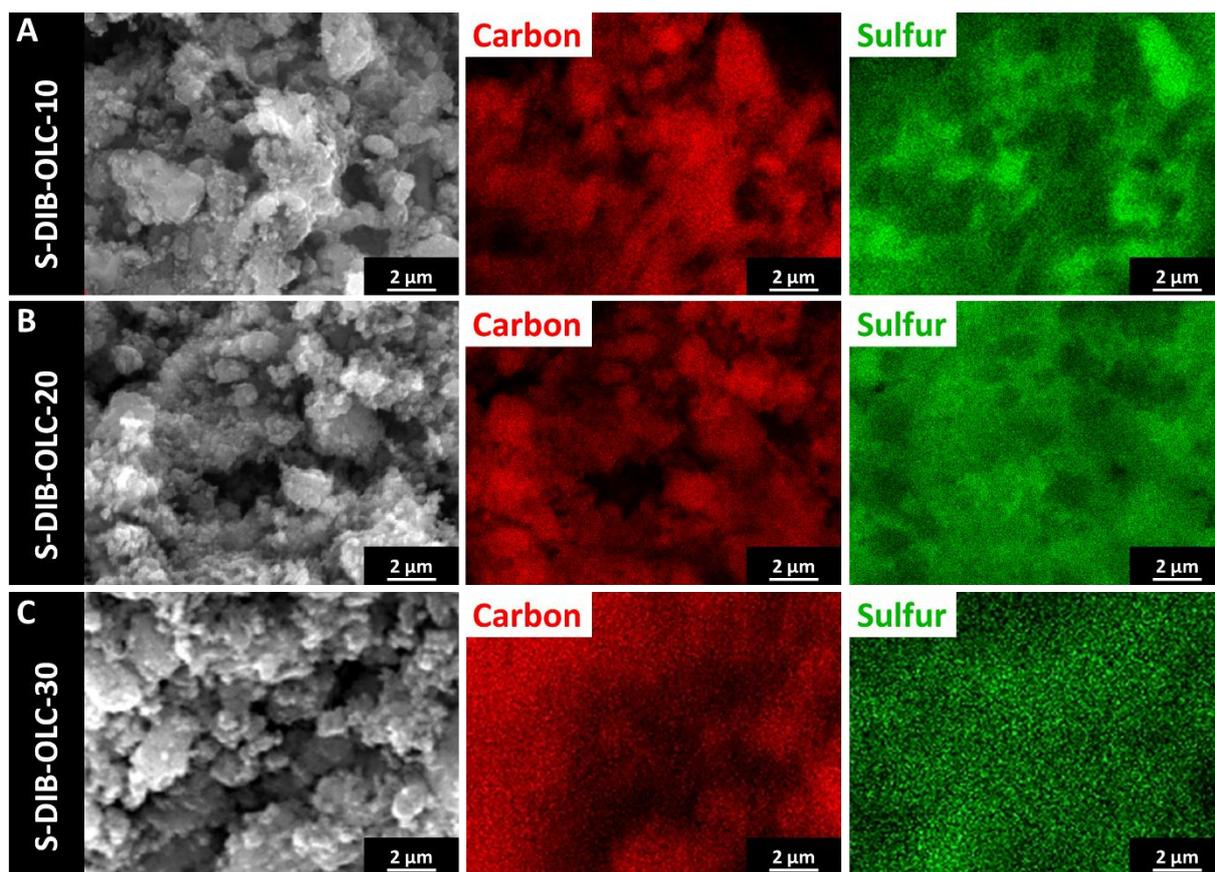
**Figure S4:** Scanning electron micrographs of carbon onion / sulfur copolymer hybrids and their corresponding elemental EDX mappings.
