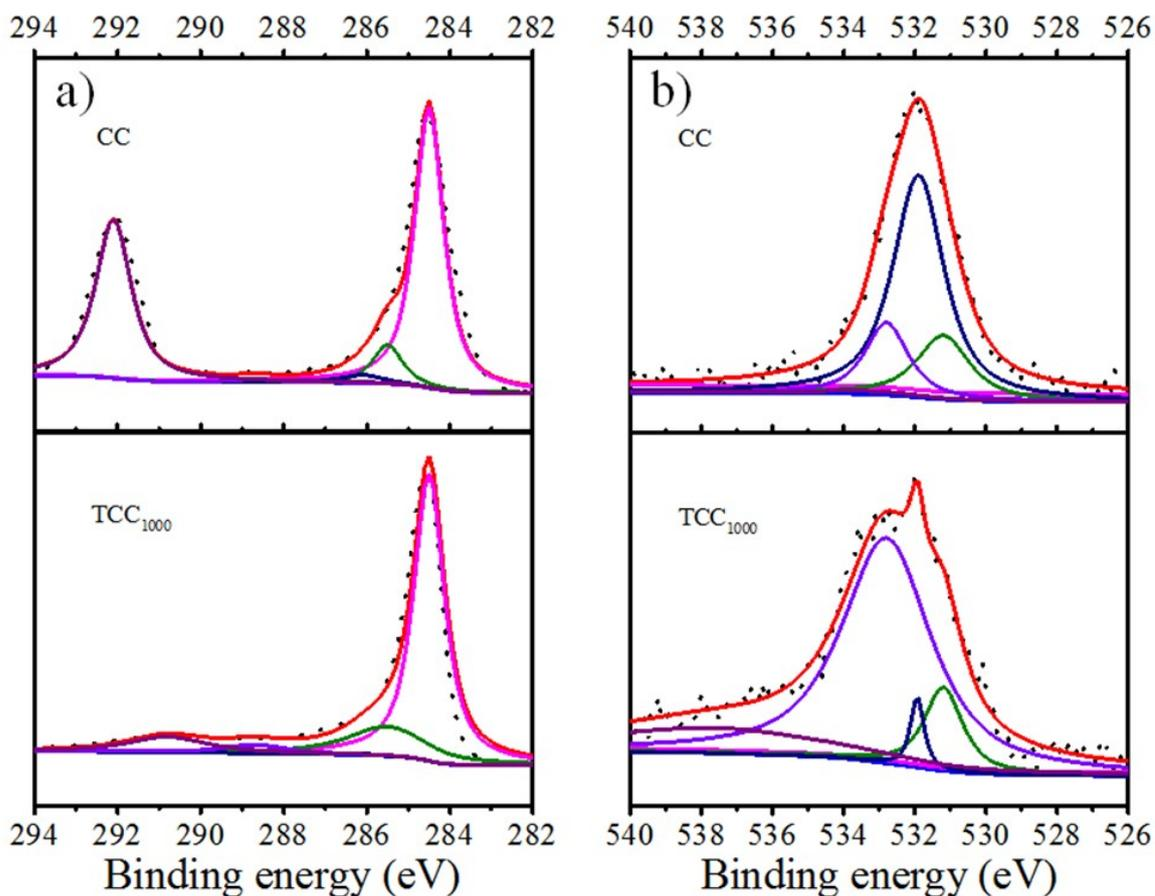
**Figure S7.** (a) The C1s and (b) O1s XPS fine scan spectrum of CC and TCC<sub>1000</sub>.
