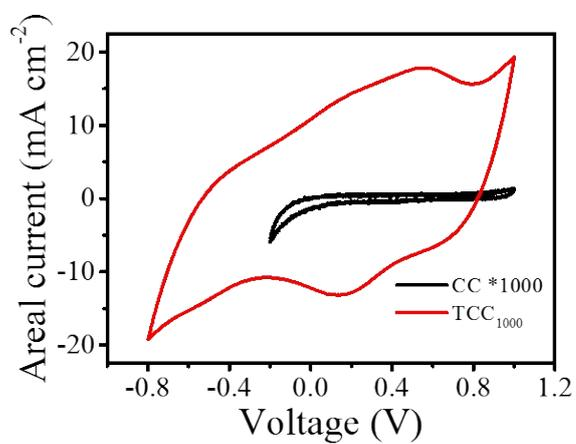
**Figure S2.** CV curves for CC (expanded for 500 times) and TCC<sub>1000</sub> in 1 M H<sub>2</sub>SO<sub>4</sub>.
