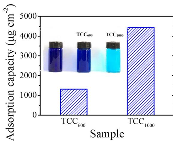
**Figure S4.** The adsorption capacity of TCC<sub>x</sub>.
