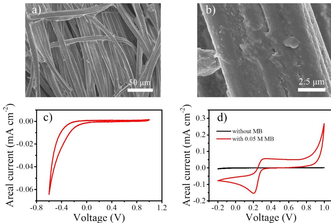
**Figure S1.** a) and b) SEM image of the CC. c) The CV curves of CC at -0.6 v-1 v in 1 M H<sub>2</sub>SO<sub>4</sub> at 5 mv s<sup>-1</sup>. d) The CV curves of CC in 1 M H<sub>2</sub>SO<sub>4</sub> with or without MB at -0.2 v-1 v at 5 mv s<sup>-1</sup>.
