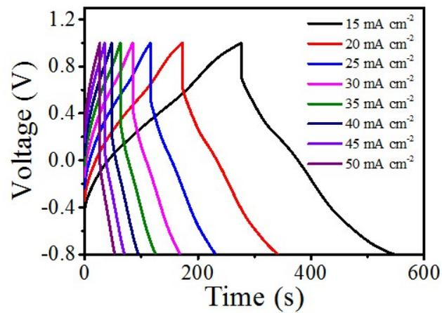
**Figure S3.** GCD curves for TCC<sub>1000</sub> in 1 M H<sub>2</sub>SO<sub>4</sub>.
