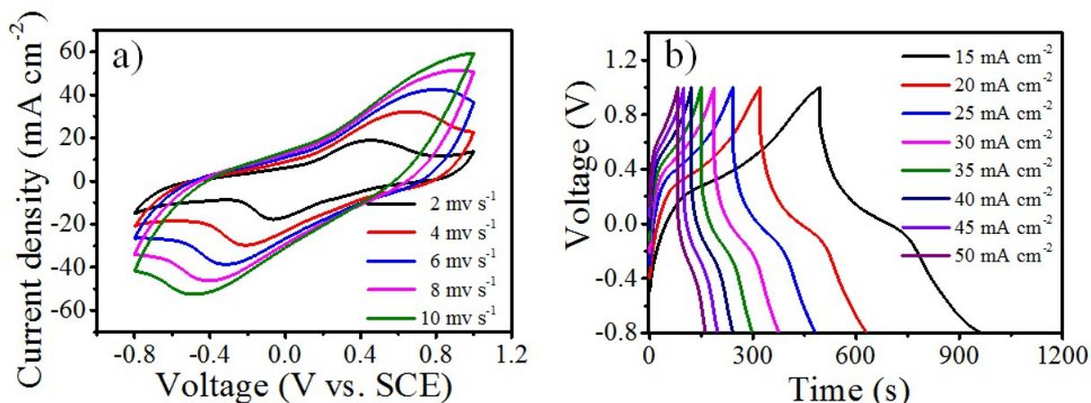
**Figure S9.** a) CV curves for TCC<sub>1000</sub> in 1 M H<sub>2</sub>SO<sub>4</sub> with 0.05 M MB. b) The GCD curves of 0.05 M MB at current densities from 15 to 50 mA cm<sup>-2</sup>.
