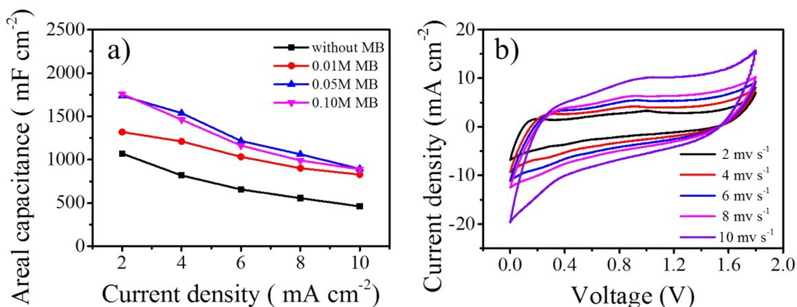
**Figure S10.** (a) Plots of the areal capacitance vs. current density for solid-state supercapacitors. (b) The CV curves of PVA-H<sub>2</sub>SO<sub>4</sub> with 0.05 M MB at different scan rates.
