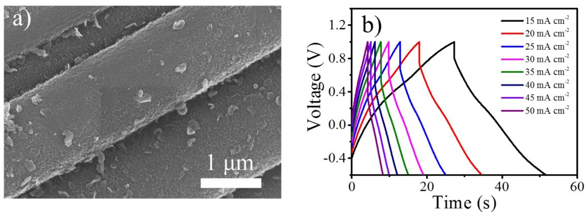
**Figure S5.** a) SEM image of the TCC<sub>600</sub>. b) The GCD curves of TCC<sub>600</sub> at -0.6-1 v in 1 M H<sub>2</sub>SO<sub>4</sub> with 0.05 M MB. Because TCC<sub>600</sub> with or without MB tested at -0.8-1 v occurred with hydrogen evolution reaction, we chose data tested at -0.6-1 v to compare with TCC<sub>1000</sub>'s in the article.
