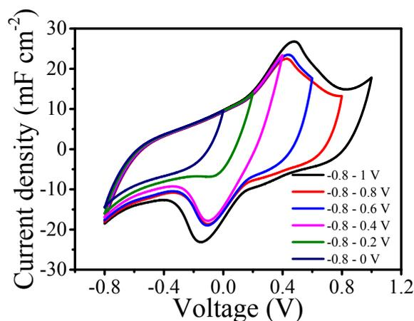
**Figure S8.** CV curves measured at different voltages at a scan rate of 5 mV s<sup>-1</sup>.
