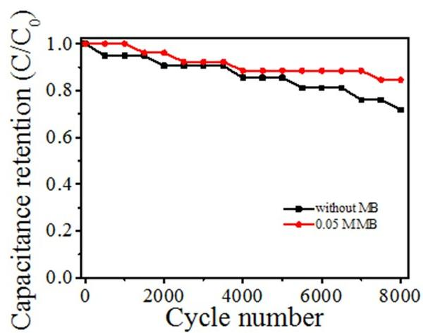
**Figure S13.** Cyclic life of PVA- $H_2SO_4$  with or without 0.05 M MB.
