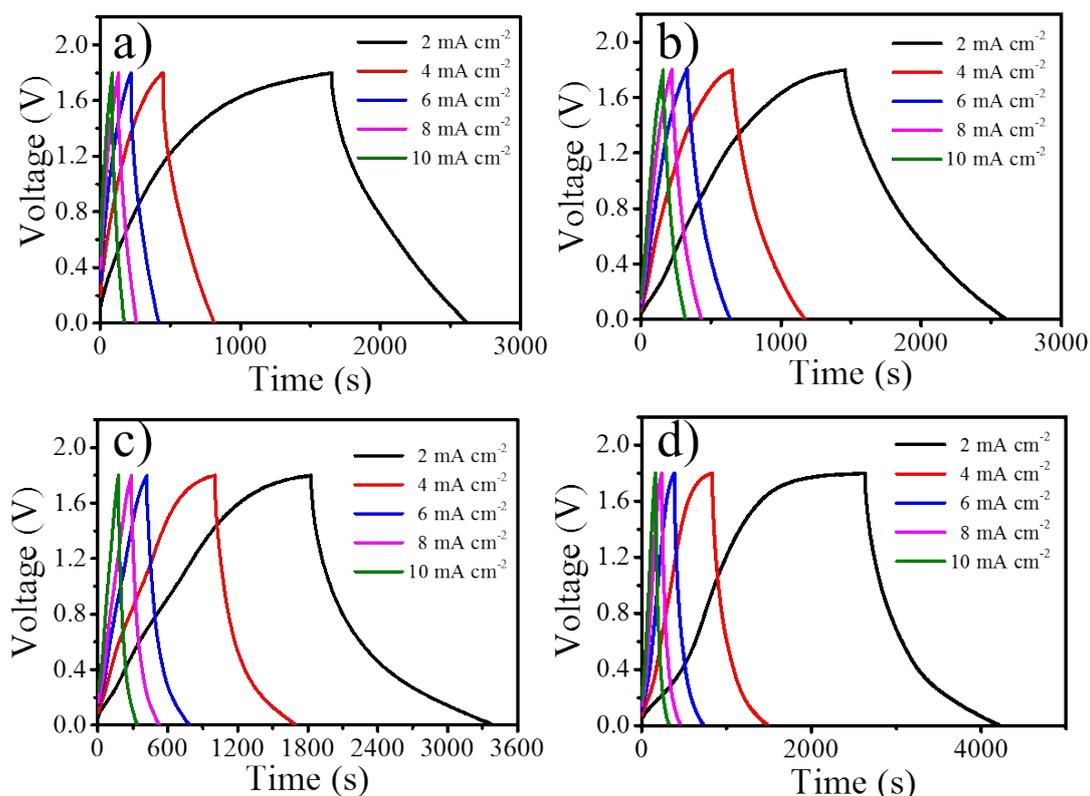
**Figure S11.** a) The GCD curves of solid-state SCs without MB. b) The GCD curves of solid-state SCs with 0.01 M MB. c) The GCD curves of solid-state SCs with 0.05 M MB. d) The GCD curves of solid-state SCs with 0.1 M MB.
