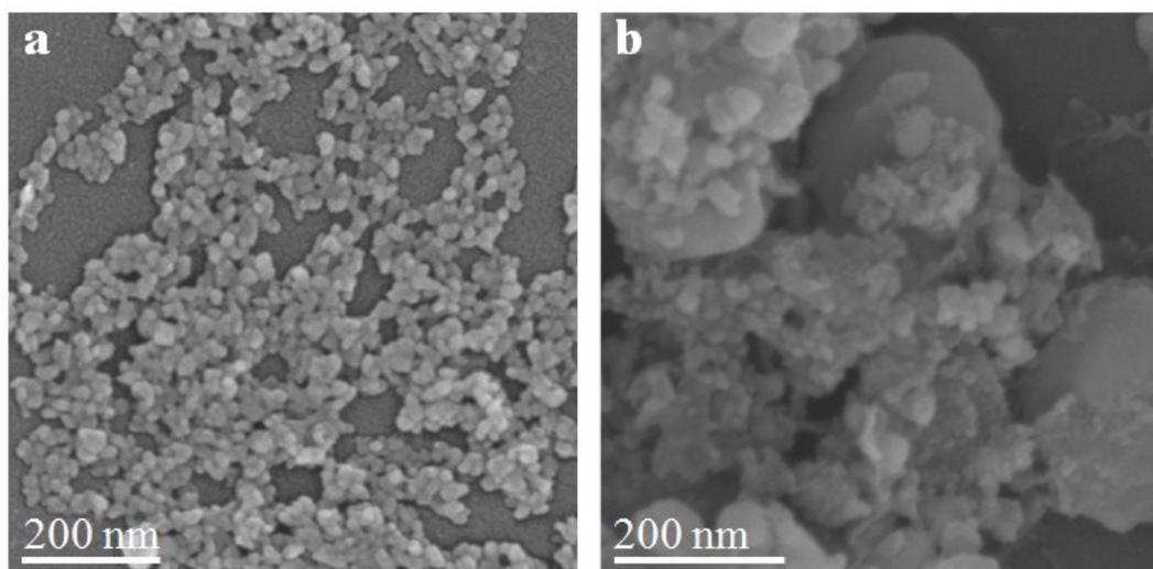
**Fig. S5** The SEM images of (a) NiFe-PBAs and (b) NiFeO<sub>x</sub>@NiFe-P. Both of NiFe-PBAs and NiFeO<sub>x</sub>@NiFe-P were produced without addition of PVP.
