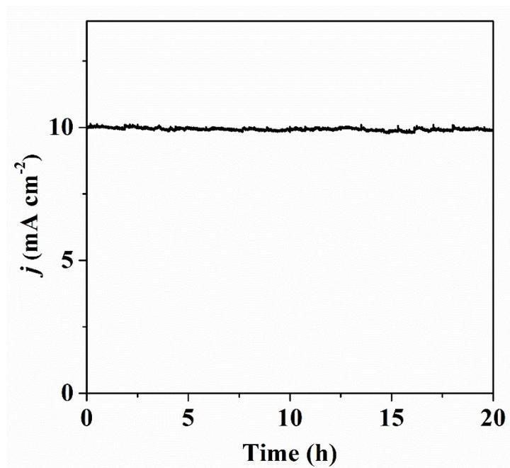
**Fig. S8** Time-dependent current density curve for NC-NiFeO<sub>x</sub>@NiFe-P catalyst at fixed potential of 1.53 V.
