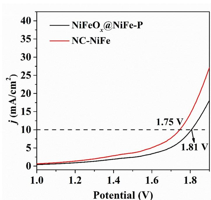
**Fig. S13** LSV of water electrolysis based on the NiFeO<sub>x</sub>@NiFe-P and NC-NiFe catalyst in 1 M KOH
