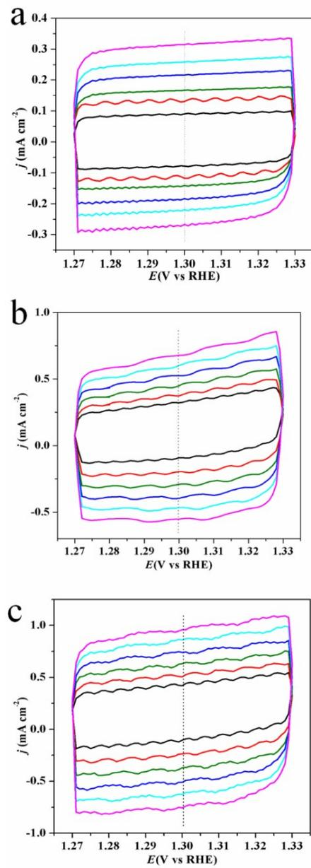
**Fig. S9** CV curves for (a)  $\text{NiFeO}_x@/\text{NiFe-P}$ , (b) NC-NiFe and (c) NC-NiFeO<sub>x</sub>@NiFe-P at various scan rates
