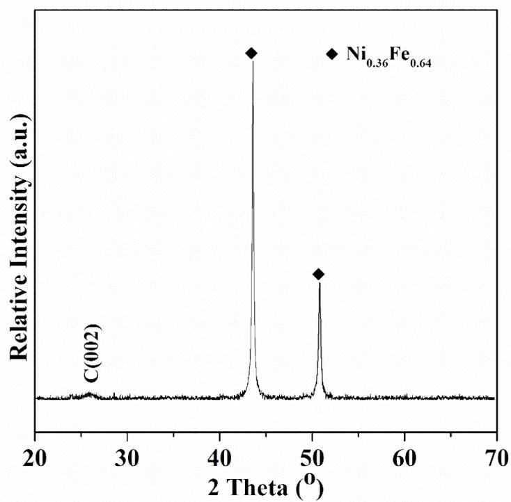
Fig. S3 The XRD pattern of NC-NiFe (served as control sample). The NC-NiFe was produced without phosphorization.
