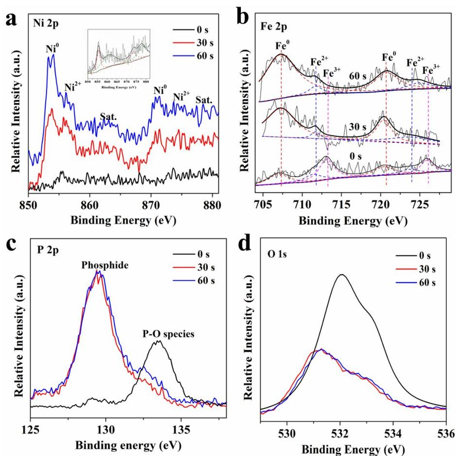
**Fig. S7** XPS spectra of (a) Ni 2p, (b) Fe 2p, (c) P 2p, and (d) O 1s for NC-NiFeO<sub>x</sub>@NiFe-P catalyst after Ar ions etching of different time (i.e. 0 s, 30 s, 60 s). The insert in (a) displayed the magnified spectrum of untreated NC-NiFeO<sub>x</sub>@NiFe-P sample
