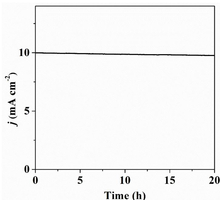
**Fig. S10** Time-dependent current density curve for NC-NiFeO<sub>x</sub>@NiFe-P catalyst at fixed potential of -0.23 V.
