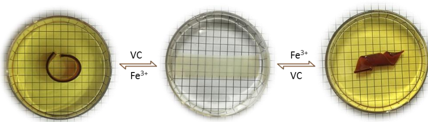
Figure S10. After immersion in vitamin C (ascorbic acid) solution, the second crosslinked network structure was erased; then transferred into \text{Fe}^{3+} solution under external stress, the previous hydrogel was reprocessed into a new geometrical shape.
