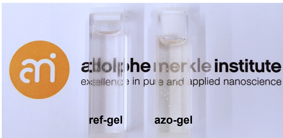
Fig. S2. Optical properties of the organogels made with PVOH of a M_w of 31-50 kDa and having a cross-link density of 10 mol%. Comparison of the visual appearance of the azo-free reference organogel ( ref-gel , left) and the azo-containing organogel ( azo-gel , right) in cuvettes.
