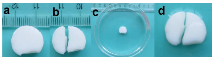
Fig. S13 Self-healing properties of H_{20} at pH 4.0: (a) original hydrogel, (b) hydrogel was cut into two pieces, (c) merged the gels by simply putting together and immersed it in PBS (pH 4.0), (d) gel after healing for 72 h at 25 °C without any external intervention.
