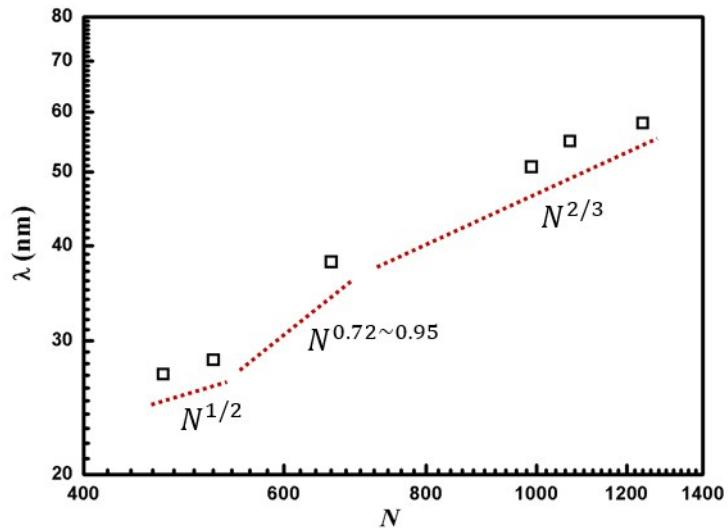
**Fig. S3** Domain spacing as a function of molecular weight for monodisperse diBCPs ( $D = 1.05 \sim 1.09$ ). The dashed red lines represent the theoretical scaling relations for weak segregation regime<sup>1</sup>, intermediate segregation regime,<sup>2,3</sup> and strong segregation regime.<sup>4</sup>
