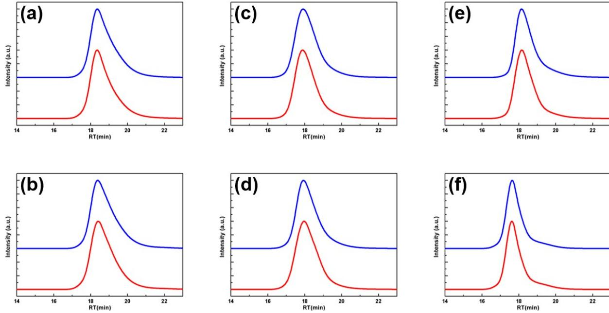
**Fig. S1** GPC traces of (a) L-ARB 60-04, (b) L-ARB 60-08, (c) L-ARB 90-04, (d) L-ARB 90-08, (e) C-ARB 80-04, and (f) C-ARB 80-08 before and after annealing. Red and blue lines represent the samples before annealing and blue lines represent the samples after annealing at 200 °C for two days.
