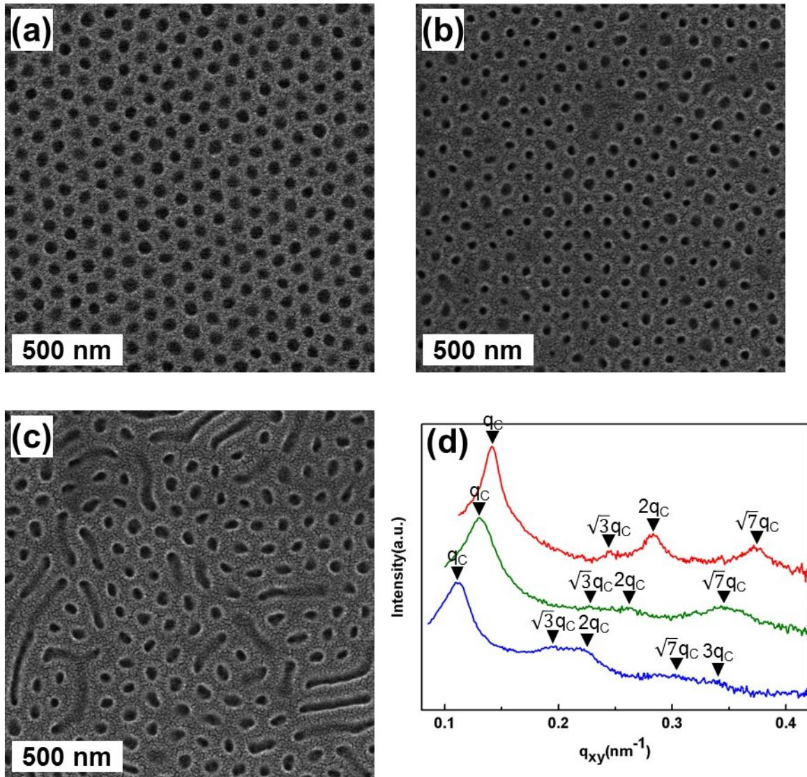
**Fig. S6** Top view SEM images of (a) C-AB 80, (b) C-ARB 80-04, (c) C-ARB 80-08 thin films, and (d) corresponding GI-SAXS profiles of these samples. Red, green, and blue lines represent C-AB 80, C-ARB 80-04, and C-ARB 80-08, respectively.
