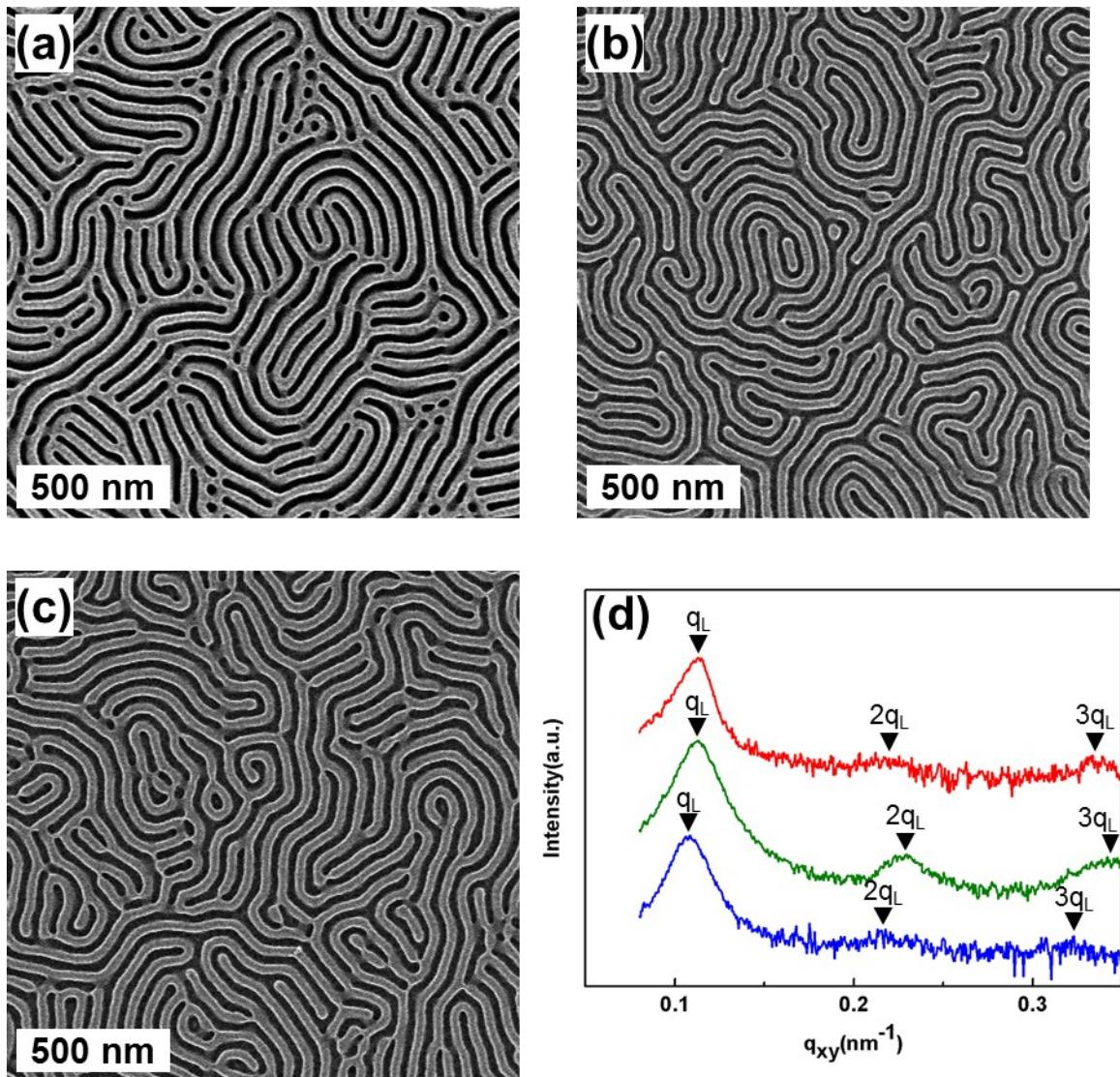
**Fig. S5** Top view SEM images of (a) L-AB 90, (b) L-ARB 90-04, and (c) L-ARB 90-08 thin films, and (d) corresponding GI-SAXS profiles of these samples. Red, green, and blue lines represent L-AB 90, L-ARB 90-04, and L-ARB 90-08, respectively.
