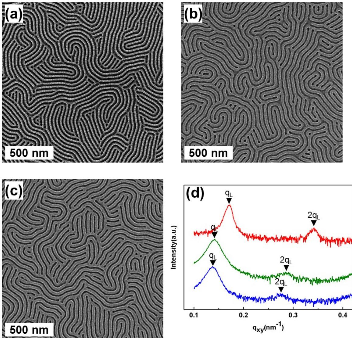
**Fig. S4** Top view SEM images of (a) L-AB 60, (b) L-ARB 60-04, and (c) L-ARB 60-08 thin films, and (d) corresponding GI-SAXS profiles of these samples. Red, green, and blue lines represent profiles for L-AB 60, L-ARB 60-04, and L-ARB 60-08, respectively.
