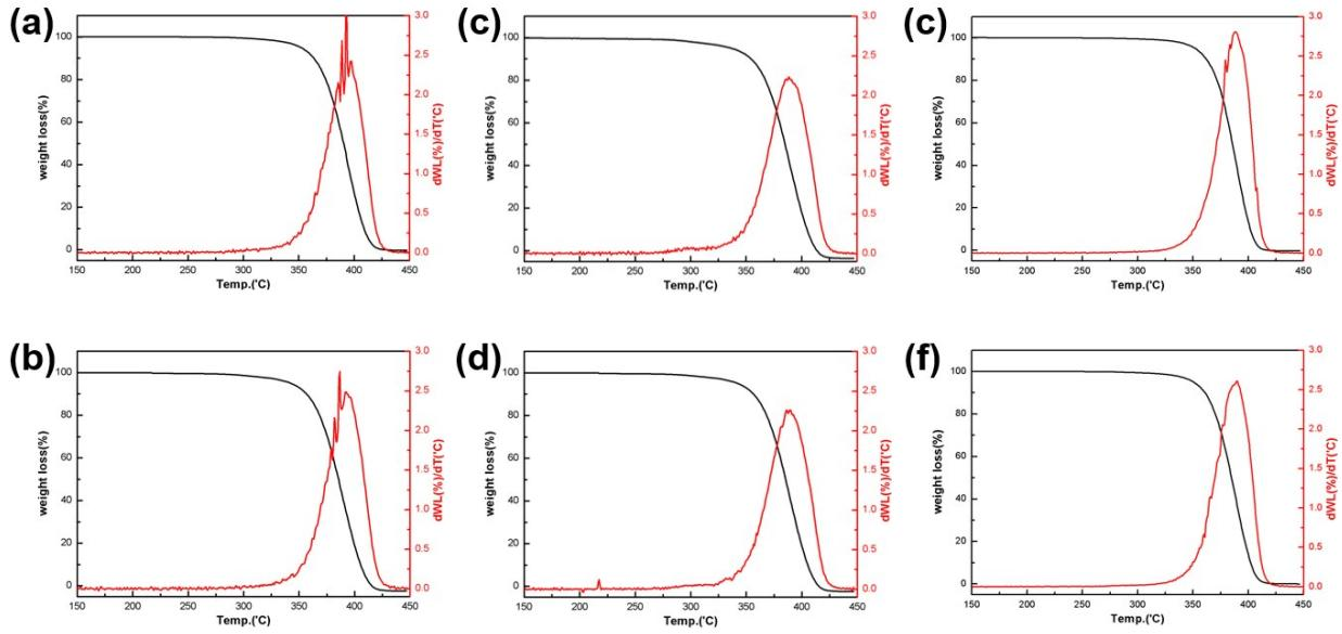
**Fig. S2** TGA traces of PS-*b*-PMMA and PS-*b*-P(S-*r*-MMA)-*b*-PMMA; (a) L-ARB 60-04, (b) L-ARB 60-08, (c) L-ARB 90-04, (d) L-ARB 90-08, (e) C-ARB 80-04, and (f) C-ARB 80-08. Black and red lines represent percentages of weight loss and TGA derivative curves as a function of temperature, respectively.
