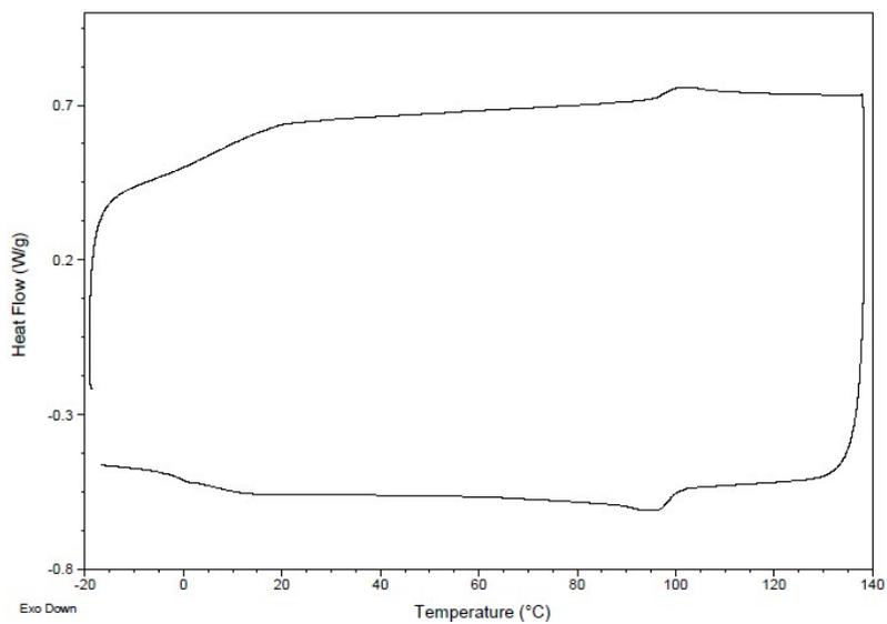
**Figure S5** DSC trace of the second heating and cooling cycle (20°C/min) for a LCE fibre.
