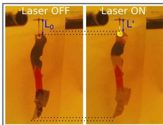
**Figure S6** Light induced contraction of a 2 mg fibre subjected to a 72 mg cargo.
