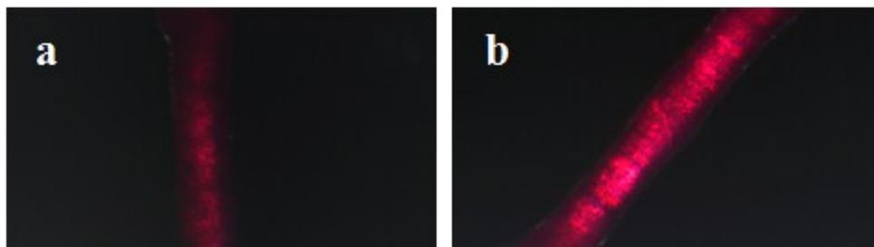
**Figure S4** POM images of a stretched fibre. Image of a fibre parallel to the cross polarizer (a) and the same fibre rotated by 45° in respect to the analyser (b).
