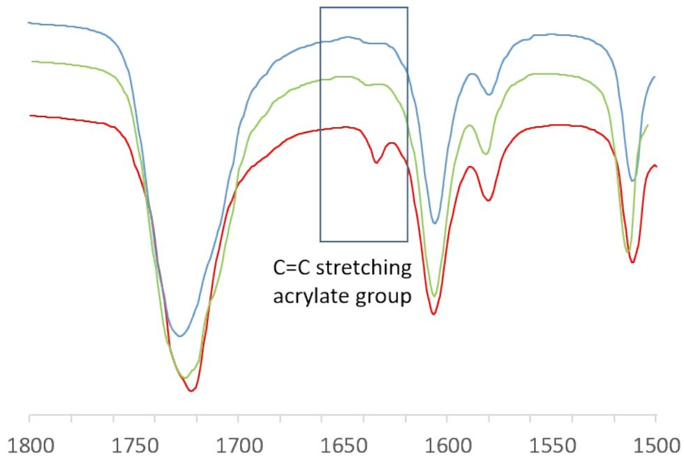
**Figure S3** ATR spectra of the monomer mixture (red line), the fibre polymerized at room temperature (green line), a fiber polymerized first at room temperature and then at 45 °C (blue line).
