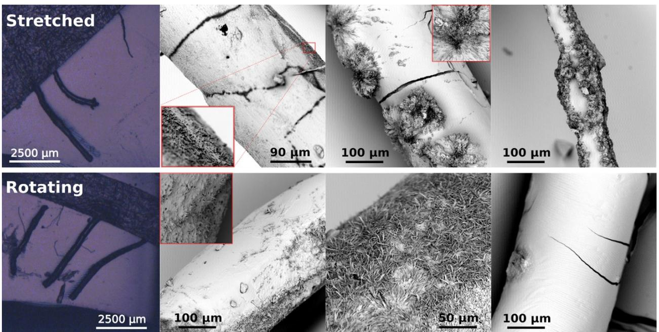
**Figure S2** Scanning electron microscope (SEM) images of a stretched (a) and a rotating fiber (b). No surface wrinkles can be associated with the two different fiber formation. Several surface formations are observed both on the stretched fiber and on the rotating one as exotic micrometric filament aggregations.
