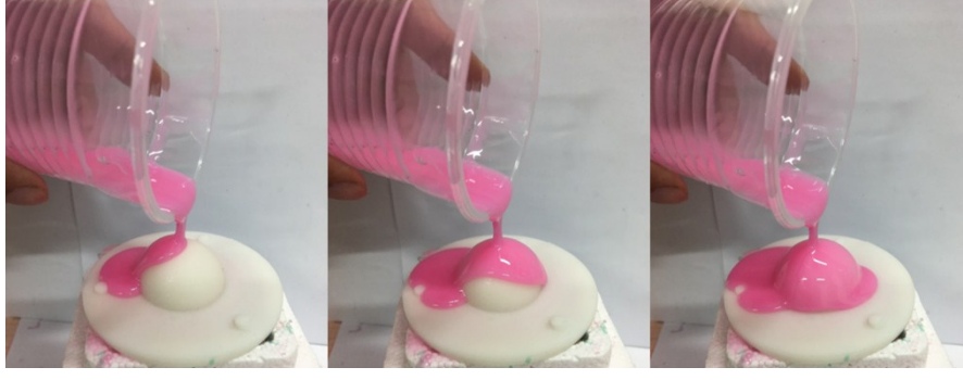
Fig. S1. Fabrication method of a hemispherical soft shell. 1
