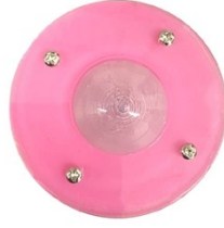
Fig. S2. Clamped boundary at the brim of the hemispherical shell.
