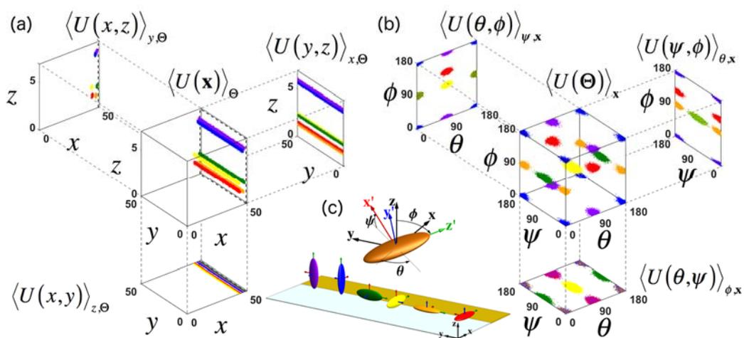
**Figure S2.** Schematic representation of coordinates for different scalene particle orientations including separated (a) positional and (b) orientational projections. (c) Schematic illustration of 6 possible orientations at the electrode edge where the electric field is a maximum. The same 6 orientations are also possible at the electrode gap center where the electric field is a minimum. Colors in part (c) correspond to the coordinates in the schematics in parts (a) and (b).
