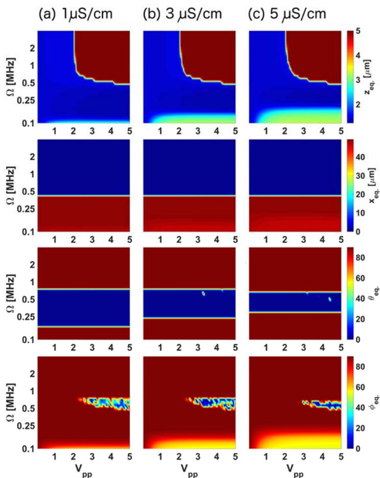
**Figure S1.** Equilibrium position and orientation of a prolate particle at different medium conductivity values (a) 1, (b) 3, and (c) 5  $\mu\text{S}/\text{cm}$ , as a function of the applied field frequency and voltage. The particle elevation has been plotted up to 5  $\mu\text{m}$  for a better representation.
