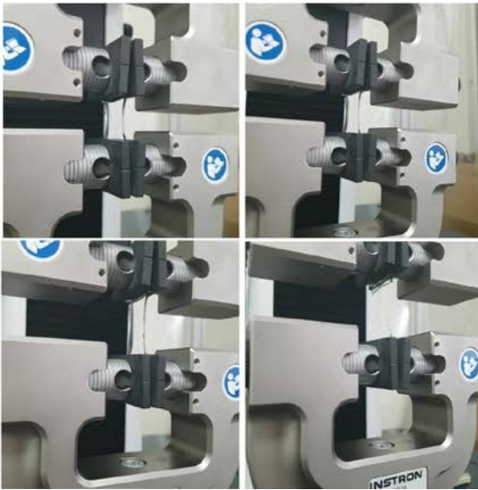
Figure S6. (a) Time lapse images of tensile test. (b) Result of tensile test.
