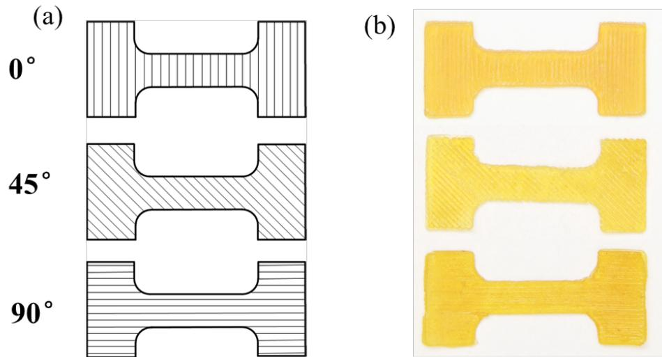
**Figure S4.** (a) and (b) the schematic illustration and the corresponding printed results of fabricated dog-bone shaped samples with different printing paths, respectively.
