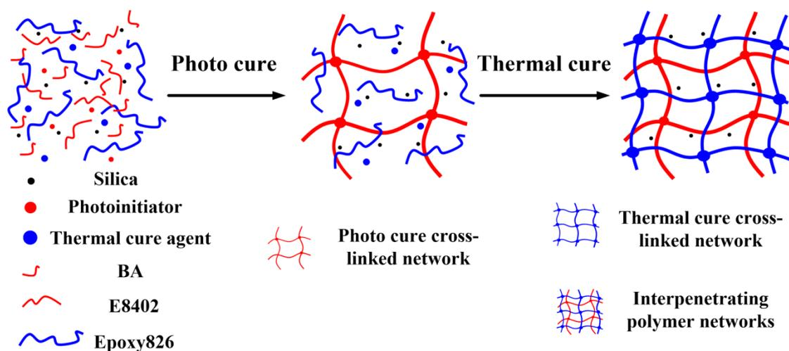
**Figure S3.** Schematic illustration of chemical reaction of the ink with two-stage cure process.
