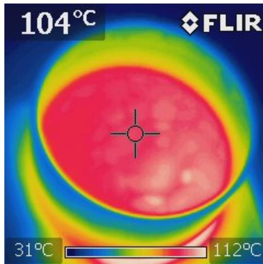
**Figure S7.** Test temperature field of pump oil bath equipped with hotplate
