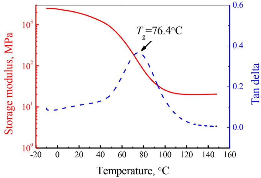
**Figure S6.** The results of thermomechanical test on the printed material.
