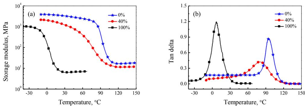
**Figure S5.** The results of DMA test on the epoxy composites with different weight fraction of photopolymer: (a) the storage modulus vs. temperature; (b) the Tan delta vs. temperature
