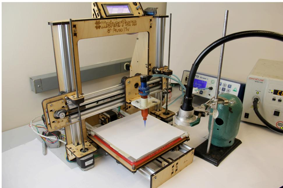
**Figure S1.** The direct ink write (DIW) set up
