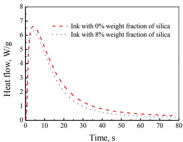
**Figure S2.** Photo-DSC curve of ink (epoxy composites with 40% weight fraction of photopolymer) with different weight fraction silica
