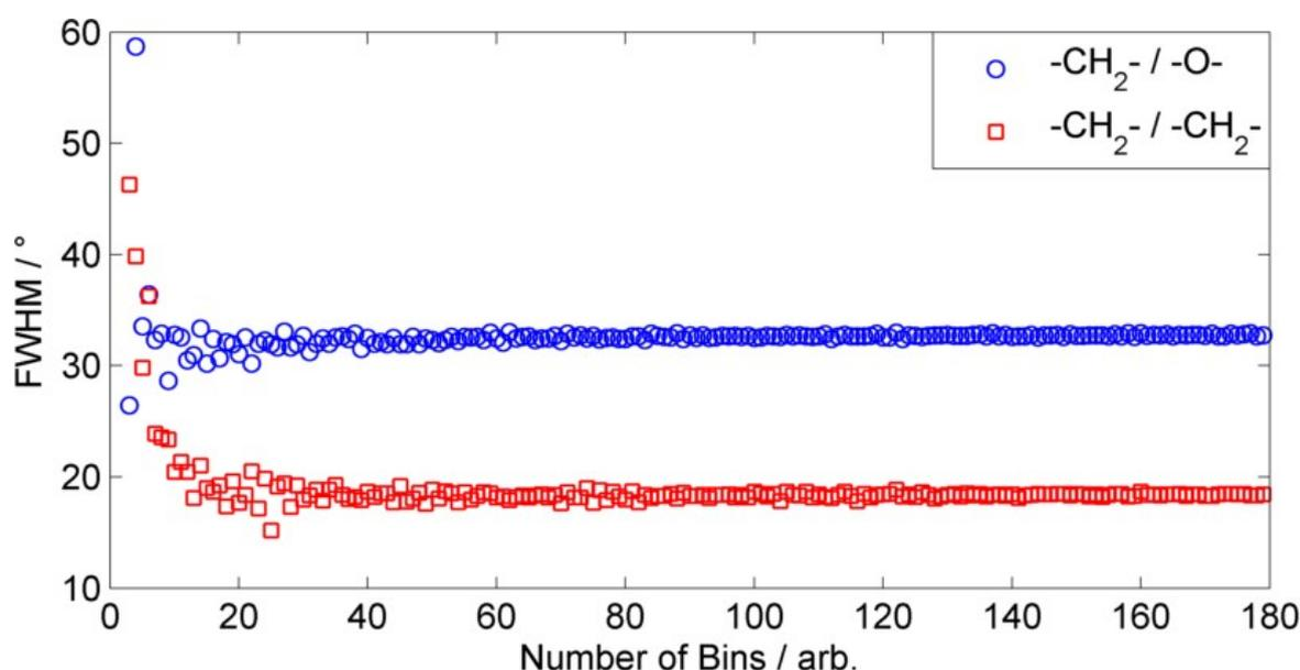
**Figure S18:** Plot of the FWHM of a Gaussian fit to histogram data (probability versus bend angle) as a function of bin size for CB9CB (-CH<sub>2</sub>-/-CH<sub>2</sub>-) and CB8OCB (-CH<sub>2</sub>-/O-).
