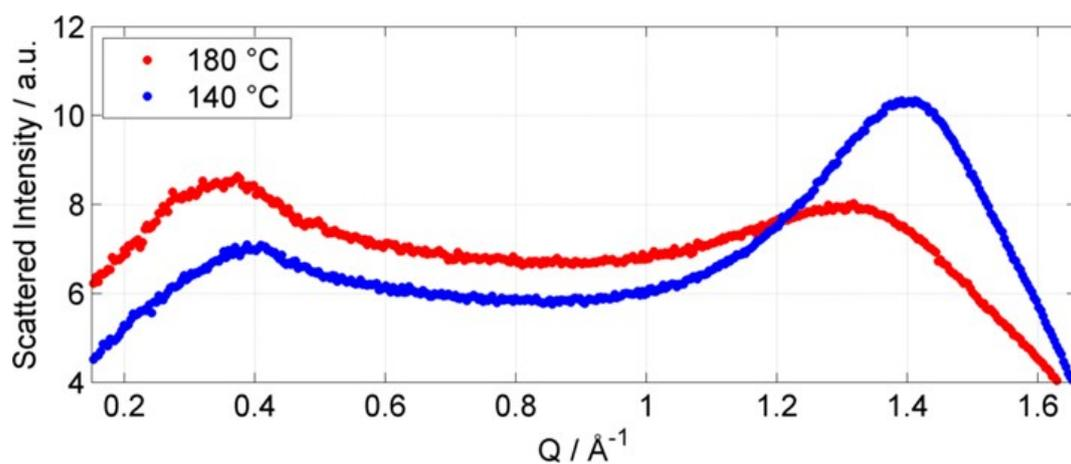
**Figure SI7:** plot of scattered intensity as a function of  $Q$  ( $\text{Å}^{-1}$ ) in both phases of compound **10** (CB8OCT) at the specified temperatures.
