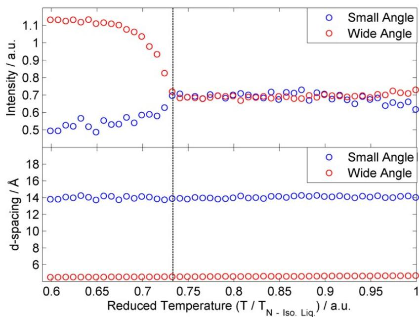
**Figure SI6:** Plot of the intensity of the small- and wide-angle peaks as a function of reduced temperature for compound **3** (top). Plot of the d-spacing (Å) of both the small- and wide-angle peaks as a function of reduced temperature for compound **3**. The dashed line corresponds to the location of the N-TB phase transition.
