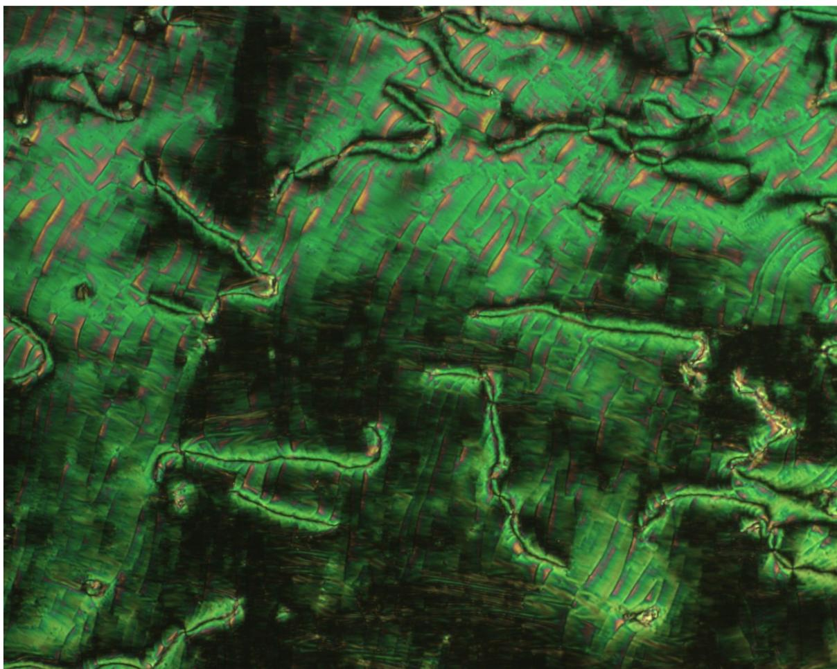
**Figure S13:** Photomicrograph (x100, crossed polarisers) of the evolution of the blocky texture of the twist-bend phase of compound **3** at 92 °C
