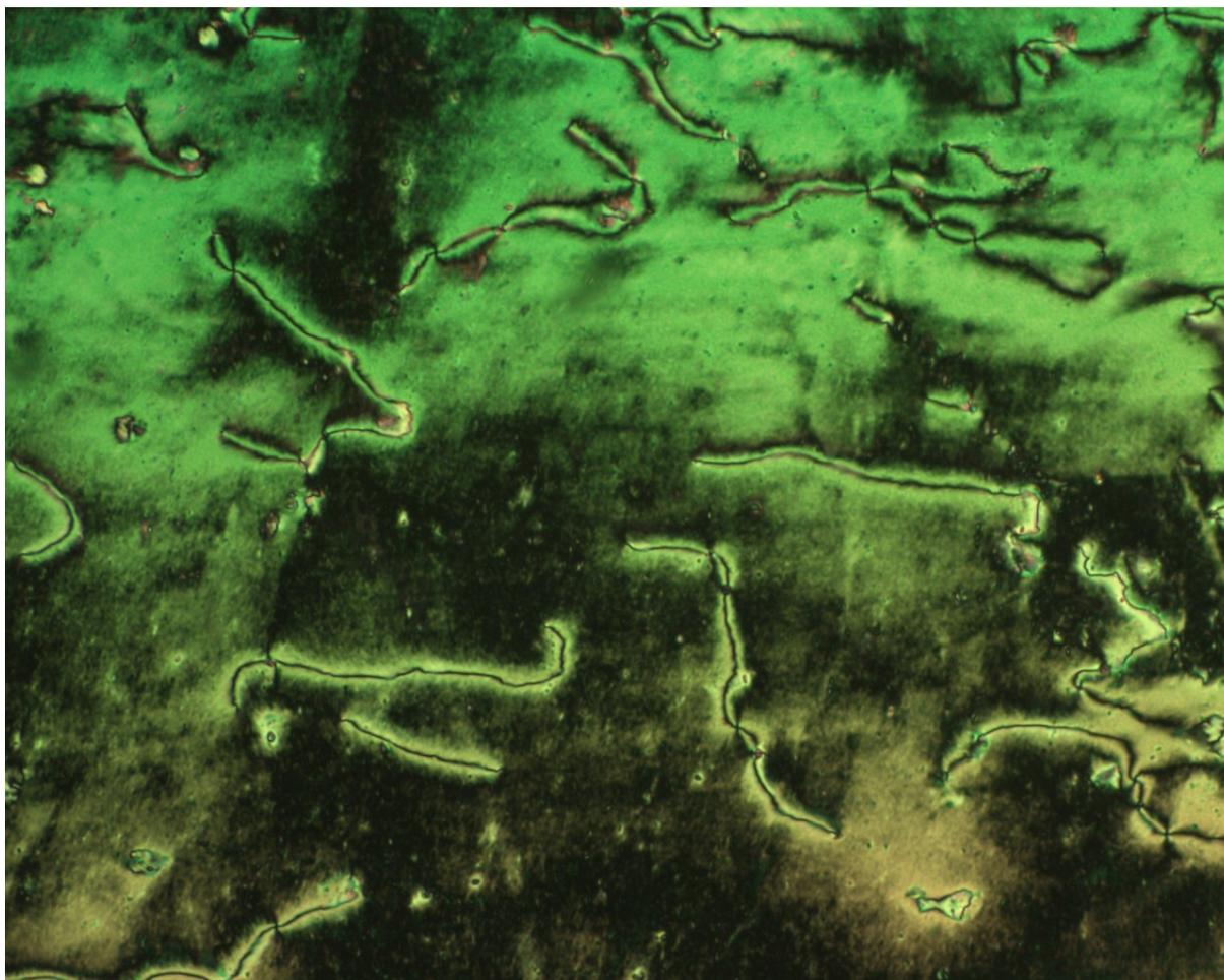
**Figure S11:** Photomicrograph (x100, crossed polarisers) of the nematic phase of compound **3** at 105 °C
