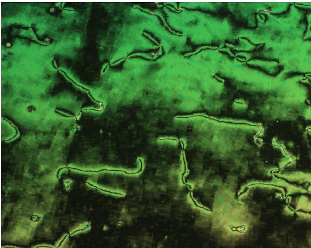
**Figure S12:** Photomicrograph (x100, crossed polarisers) of the blocky texture of the twist-bend phase of compound **3** at 94 °C
