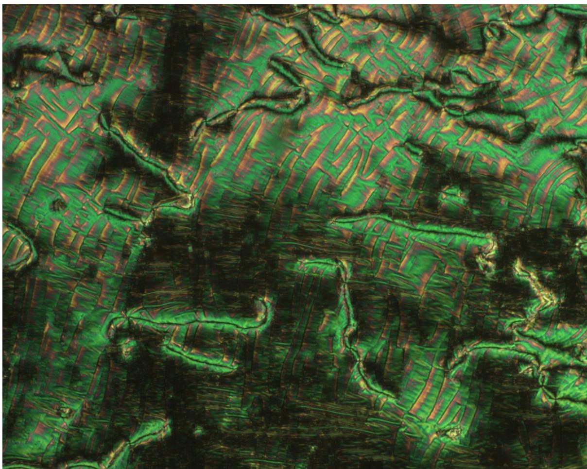
**Figure S14:** Photomicrograph (x100, crossed polarisers) of the evolution of the blocky texture of the twist-bend phase of compound **3** at 90 °C
