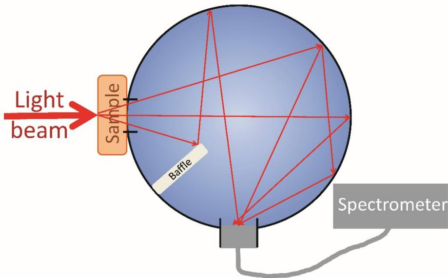
Figure S2: Schematic overview of the setup for total transmission measurements. An integrating sphere of 15 cm in diameter was used (Labsphere). The sample and light beam opening was 18 mm, the detector port opening was 3 mm.
