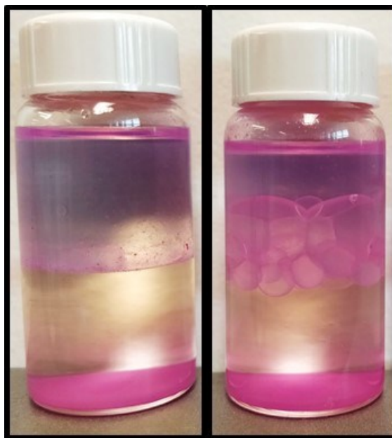
Figure S6. Images of hand shaken emulsions obtained with ~5 wt % HMDS-SNPs dispersed in the water phase before (a) and after (b) the addition of 1 g of NaCl 1 day after preparation. It can be seen here that large droplets stabilized by the HMDS-SNPs are only observed in the presence of salt when such a low energy emulsification method is used, suggesting that electrostatic repulsion governs, in part, the formation of SNP stabilized emulsions.
